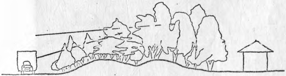
Detail No. 29 - Landscaping - Irregular Topography With Tall And Dense Vegetation Preferably On Both Sides Of Street (Sound Transmission : Motor Vehicles, Aircraft To Exterior Of House) No Scale
