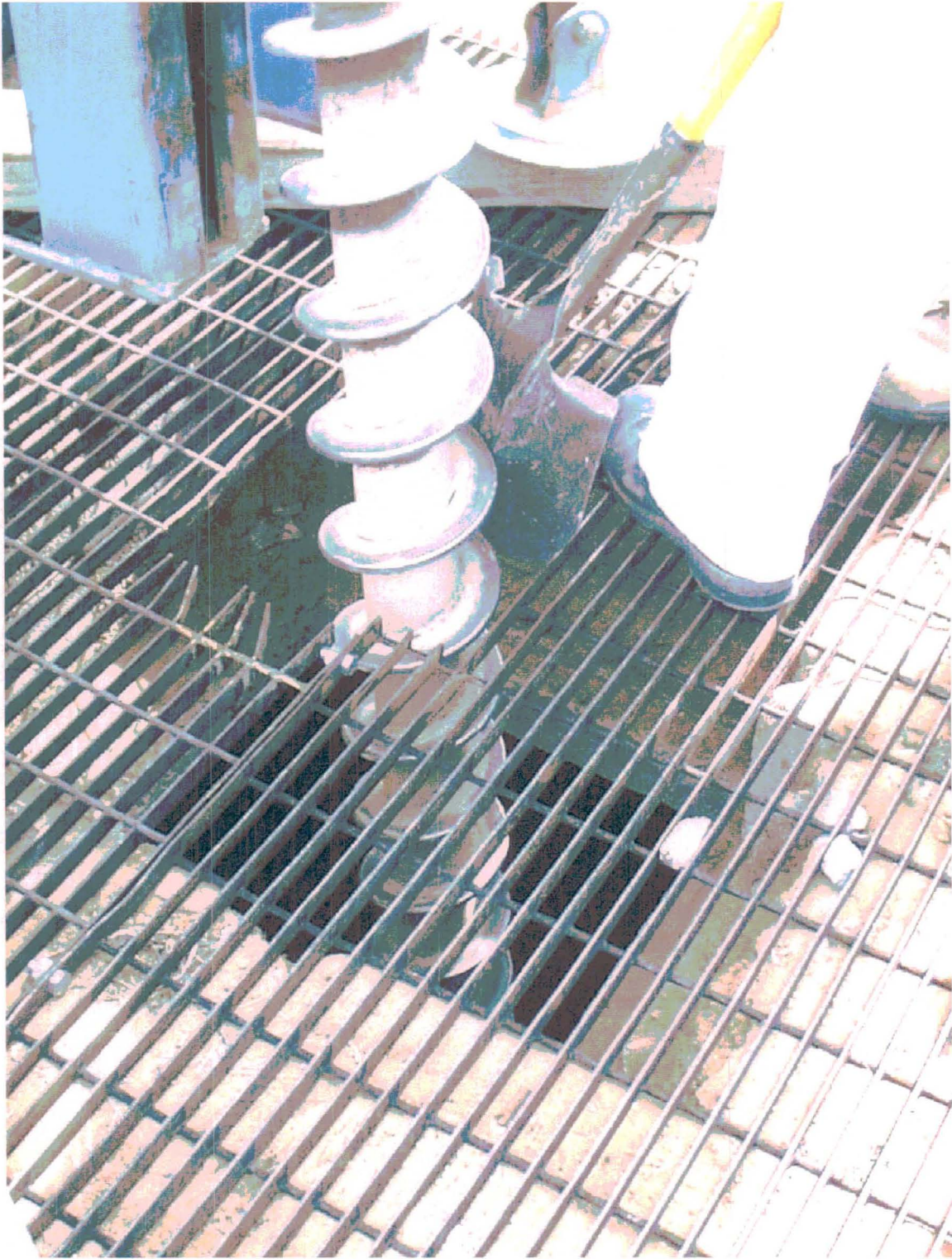
Figure 3.3-2 Collecting soil samples beneath the east seepage pit at DSS Site 1108, Building 6531. View to the northwest. September 3, 2002
