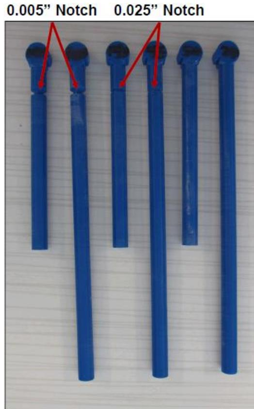
**Figure 11. Close up picture of ABS beams used in testing**
