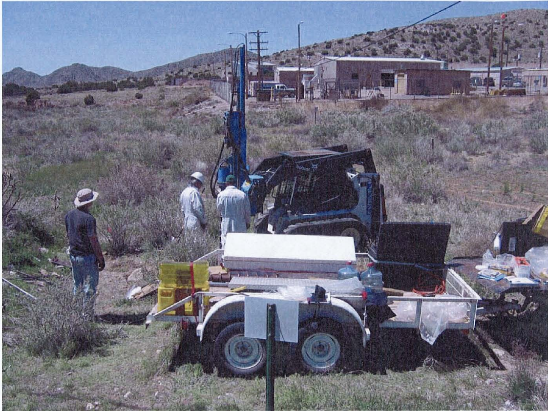
Figure 3.3-1 Collecting soil samples with the Geoprobe™ at DSS Site 1094, Live Fire Range East Septic System. View to the northwest. April 26, 2005
