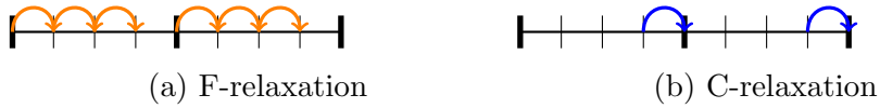
Figure 2.2: Schematic view of the action of (a) F-relaxation and (b) C-relaxation with a coarsening factor of four
