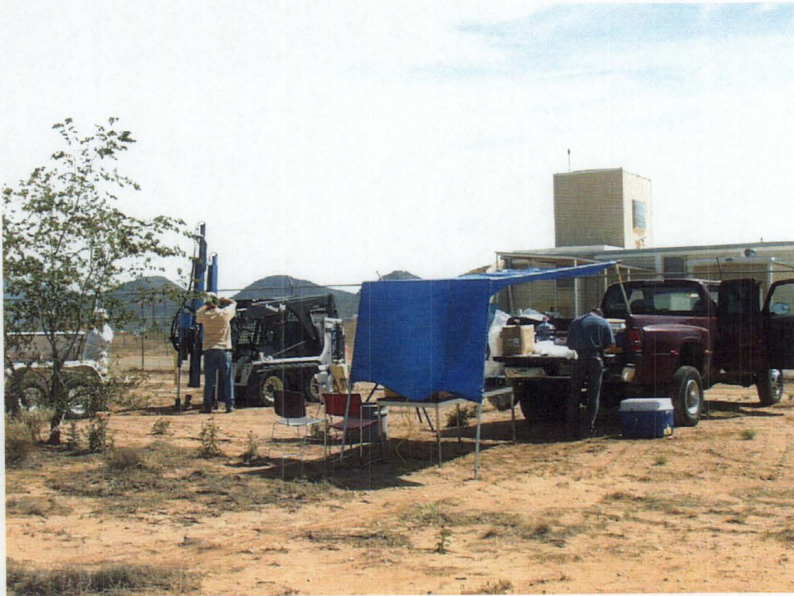
Figure 3.3-2 Collecting soil samples with the Geoprobe™ from beneath the Building 6640 Septic System drainfield, DSS Site 1078. View to the northeast. August 23, 2002
