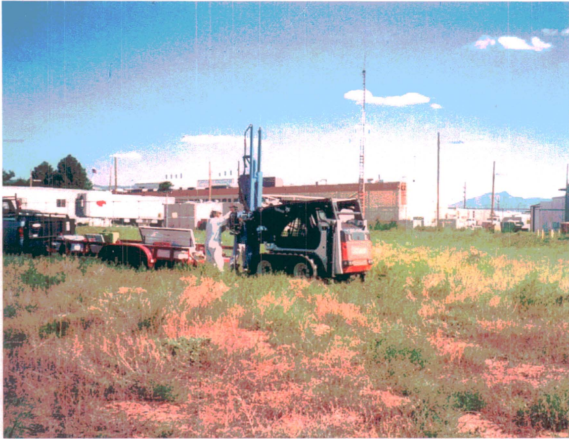
Figure 3.4-1 Collecting soil samples with the Geoprobe™ in the drainfield area of DSS Site 1029, Building 6584 North Septic System. View to the southeast. August 24, 1999
