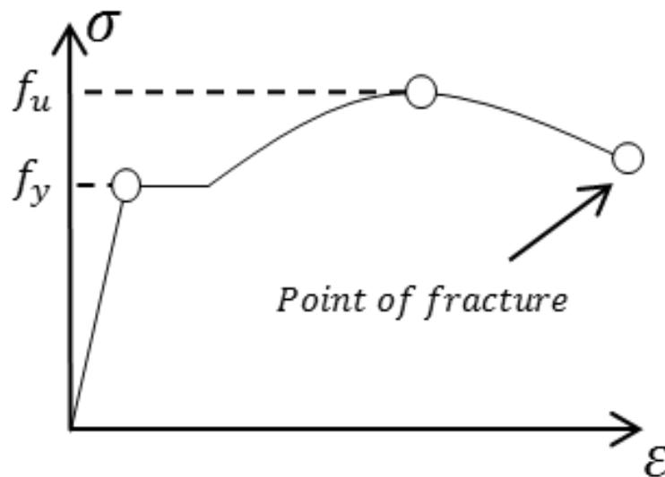
Figure 2.6: Stress-strain curve of low carbon alloy
