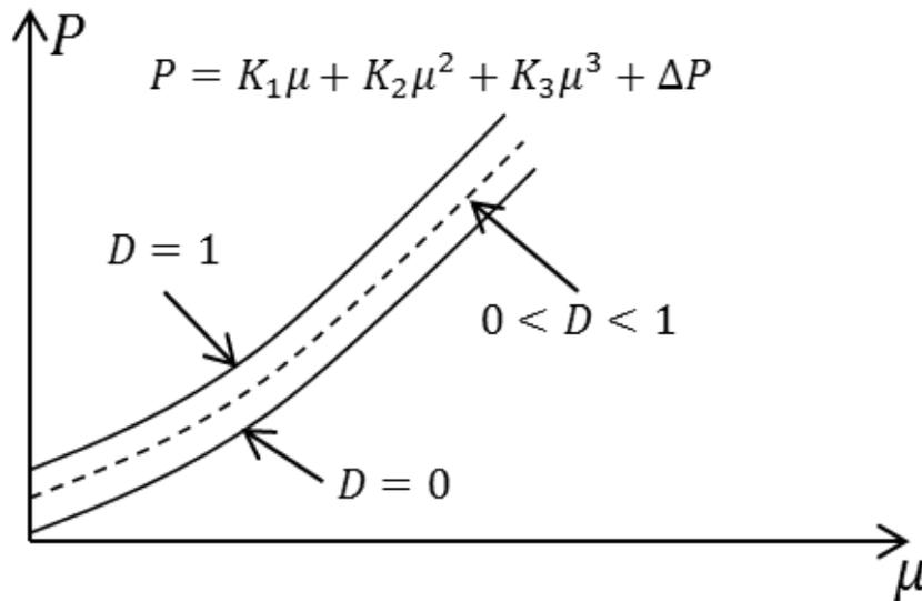
Figure 2.10: Pressure-Volumetric strain relationship for JH2
