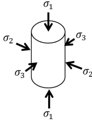
**Figure 2.3: Triaxial compression loading**
