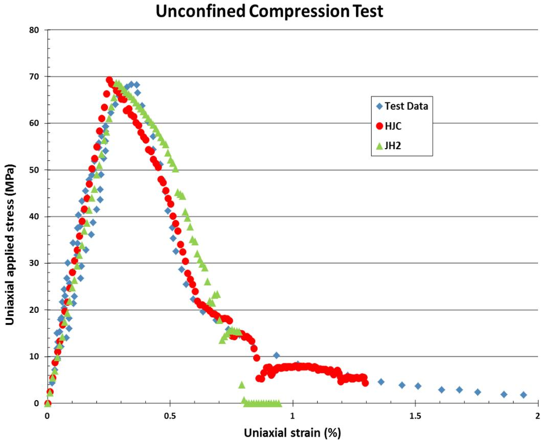
Figure 5.1: Concrete unconfined compression
