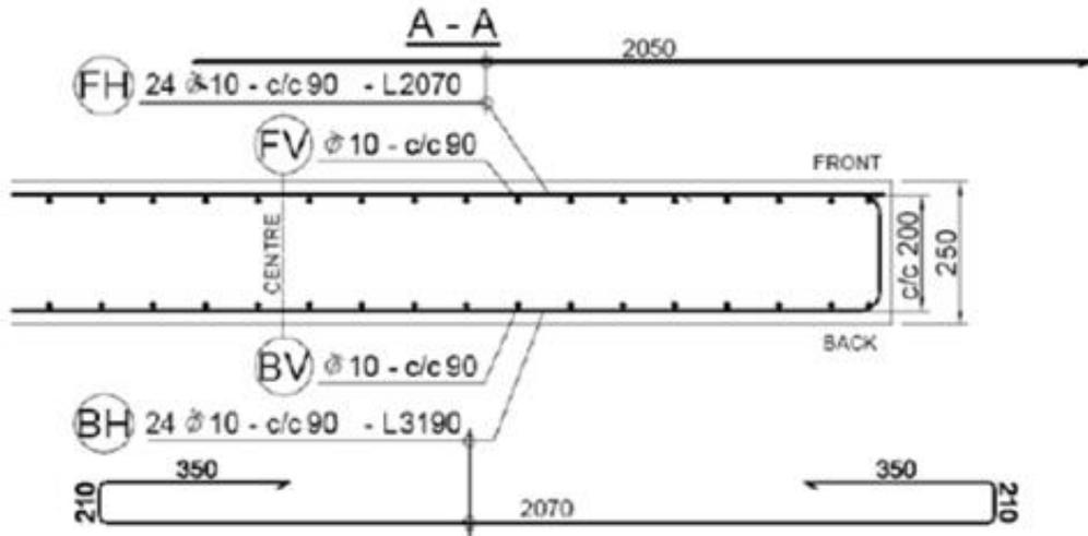
*Horizontal cross section A-A of the wall.*
