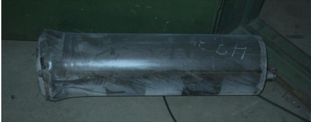
**Figure 5.35: VTT Punching solid missile post impact**
