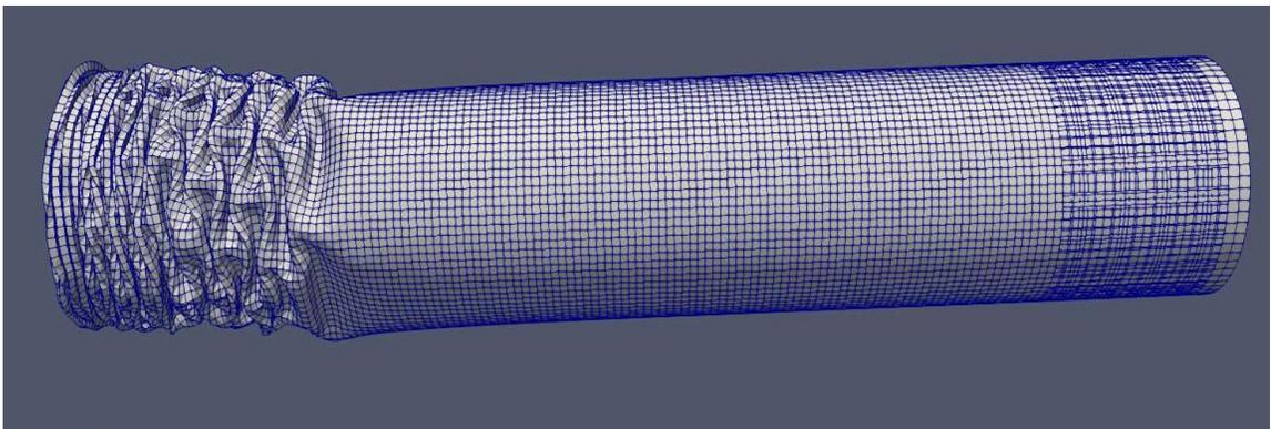
Figure 5.26: Deformed hollow missile from numerical simulation (JH2)
