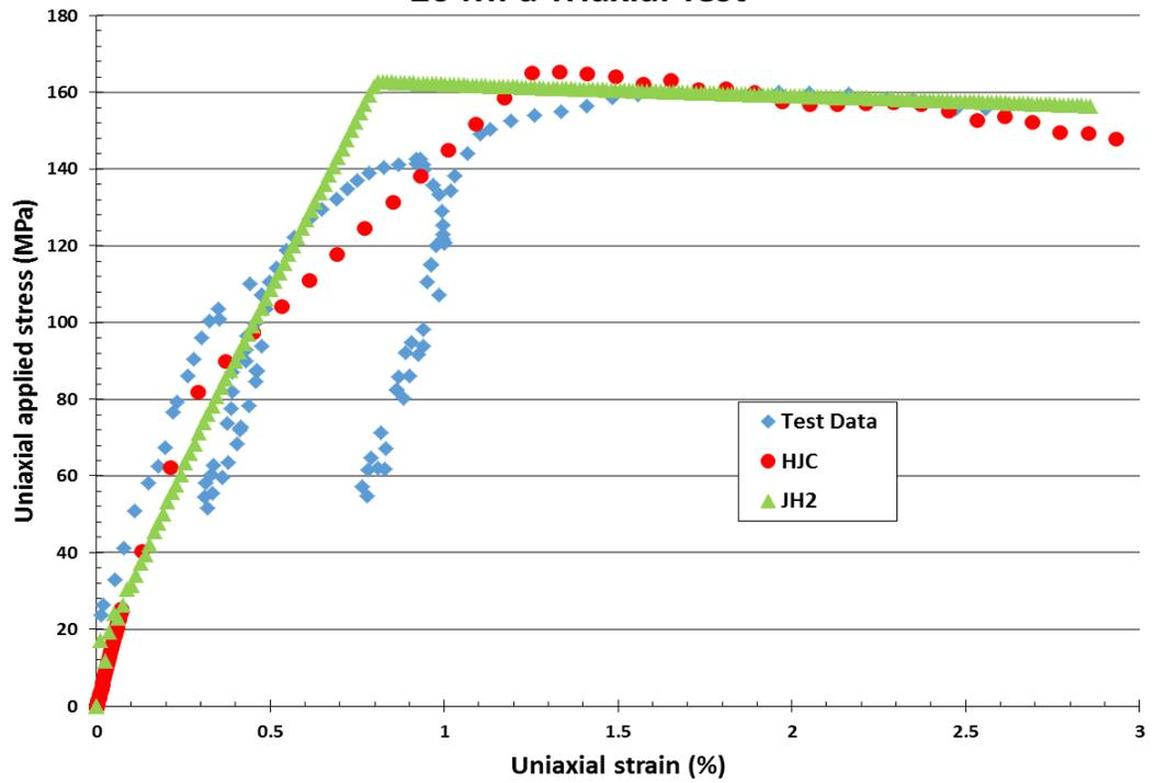
Figure 5.3: Concrete triaxial compression (26 MPa)
