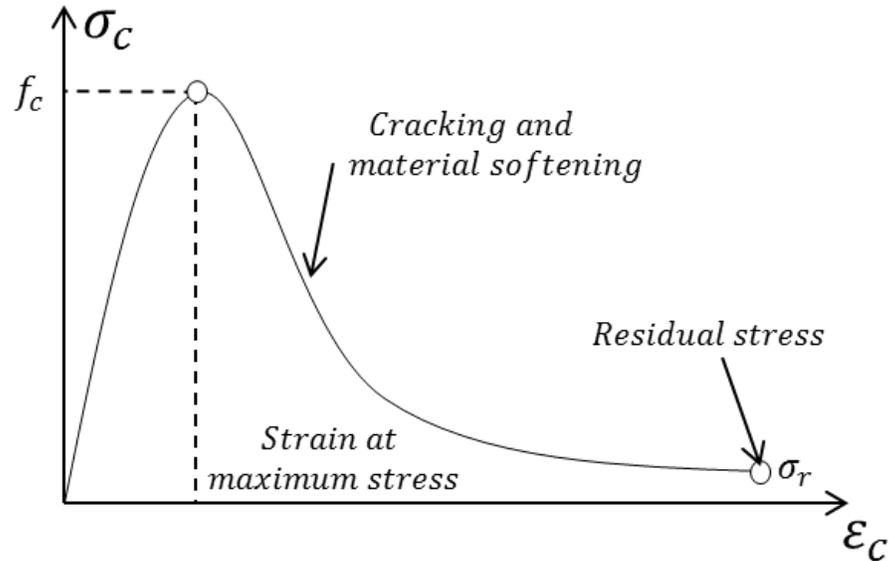
Figure 2.1: Stress-strain curve for concrete in compression
