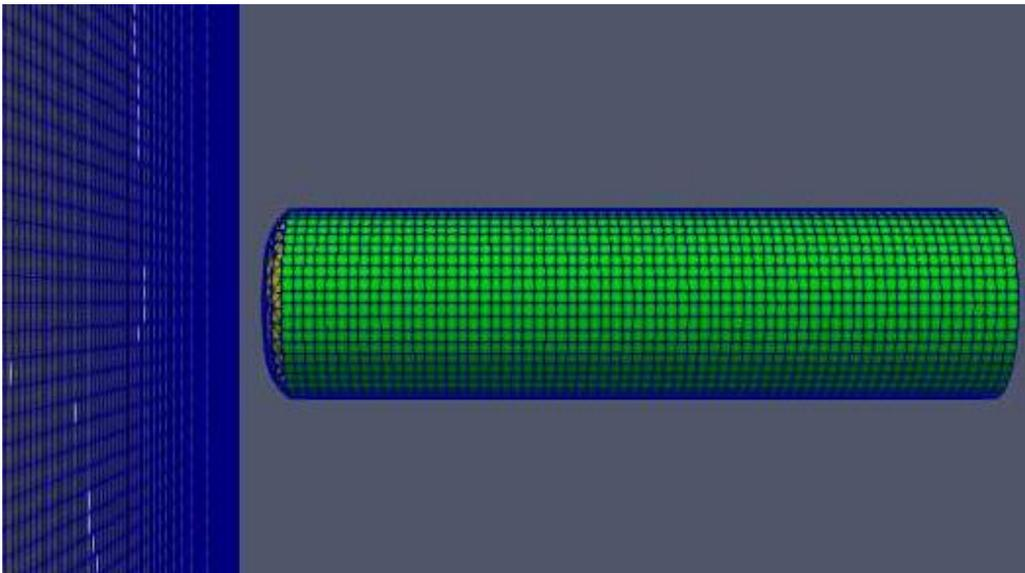
**Figure 5.34: Hex and tet element solid punching missile**
