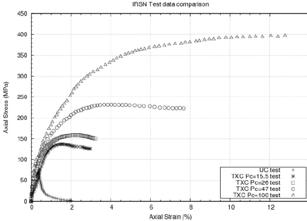
Figure 3.1: 2012 IRSN Axial stress-strain data for unconfined (UC) and Triaxial Compression (TxC) concrete specimens at varying confinement pressures
