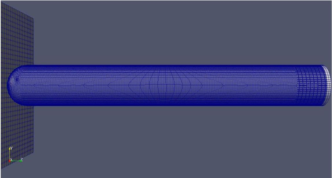
**Figure 5.7: Fine missile mesh (85,000 elements)**
