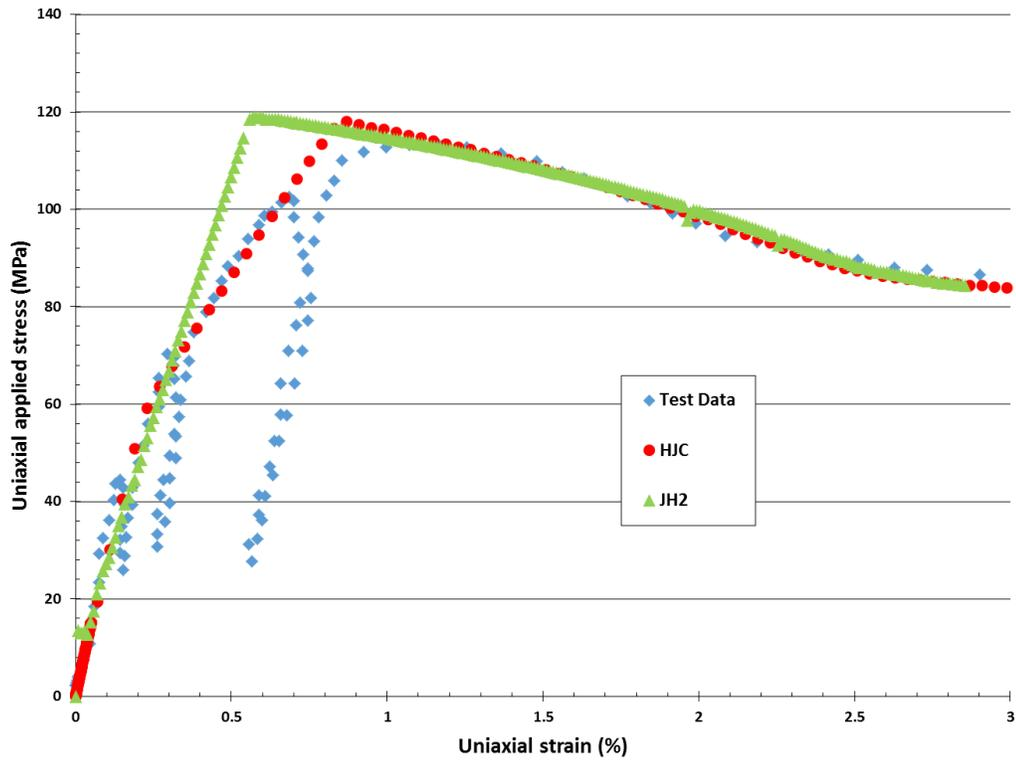
Figure 5.2: Concrete triaxial compression (15.5 MPa)
