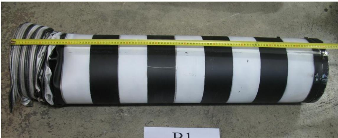
Figure 5.24: Deformed hollow missile from VTT experiment
