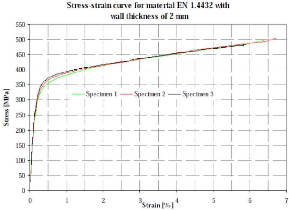
Figure 3.5: Stress-strain curve for flexural missile material EN 1.4432
