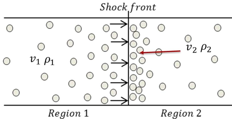
Figure 2.7: Propagating shockwave caused by ballistic impact
