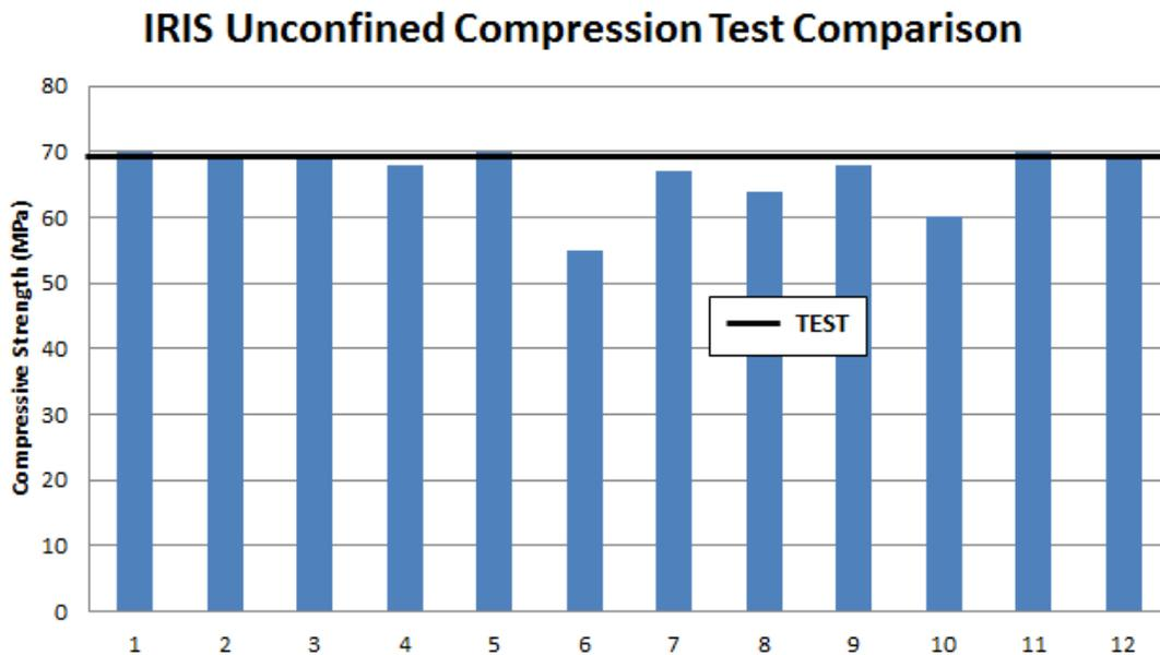
Figure 5.41: Material model unconfined compression test compressive strength comparison
