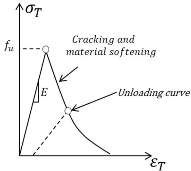
Figure 2.2: Stress-strain curve for concrete in tension
