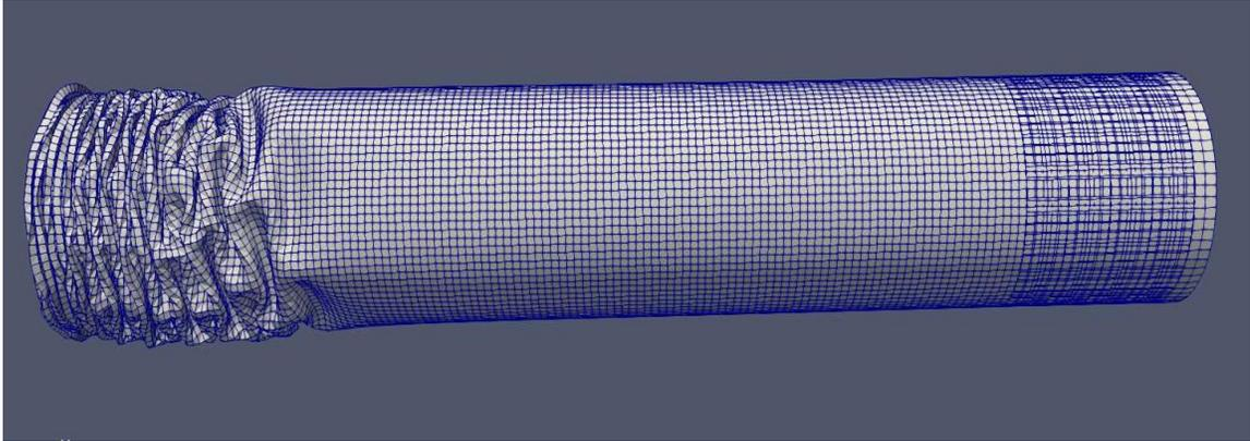
Figure 5.25: Deformed hollow missile from numerical simulation (HJC)
