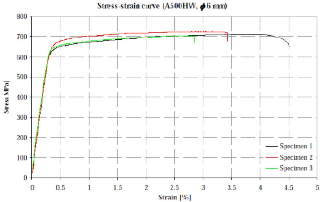
Figure 3.2: Stress-strain curve for A500HW 6mm steel rebar
