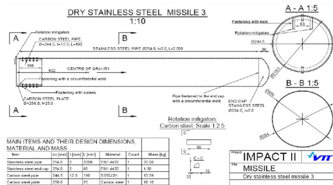
Figure 3.4: ISRN VTT flexural steel missile engineering drawing
