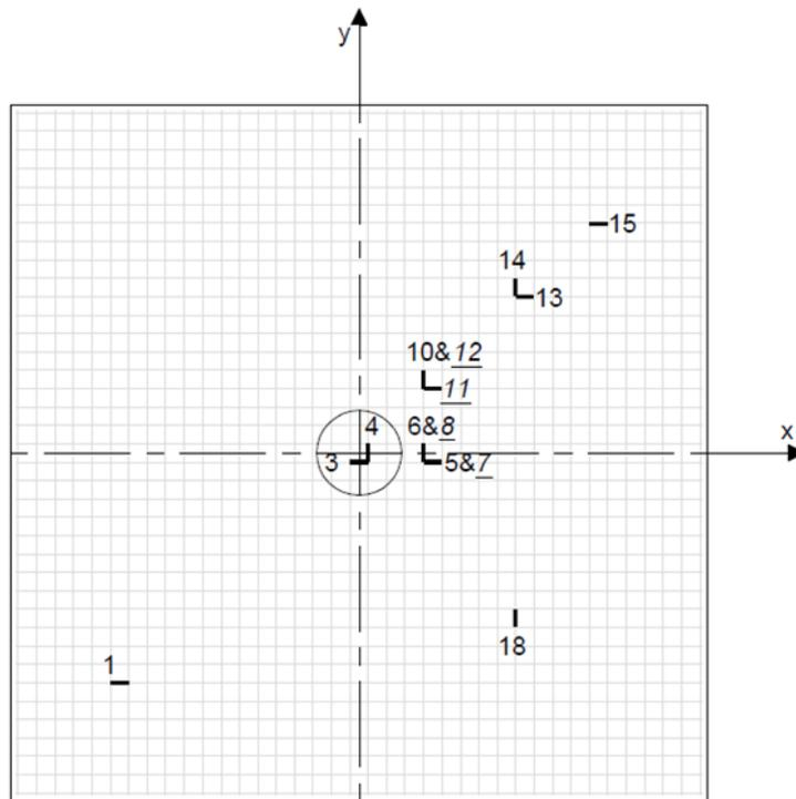
Figure 3.10: IRSN VTT Flexural rebar strain gauge locations
