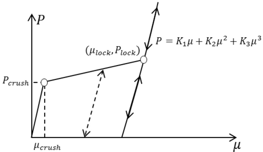
Figure 2.9: HJC hydrostatic pressure and volumetric strain relationship
