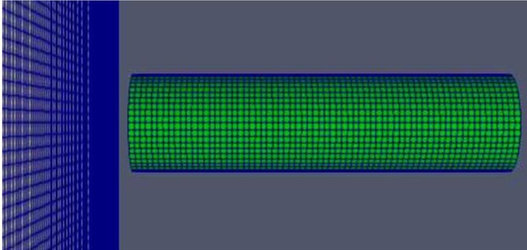
**Figure 5.33: Hex element solid punching missile**
