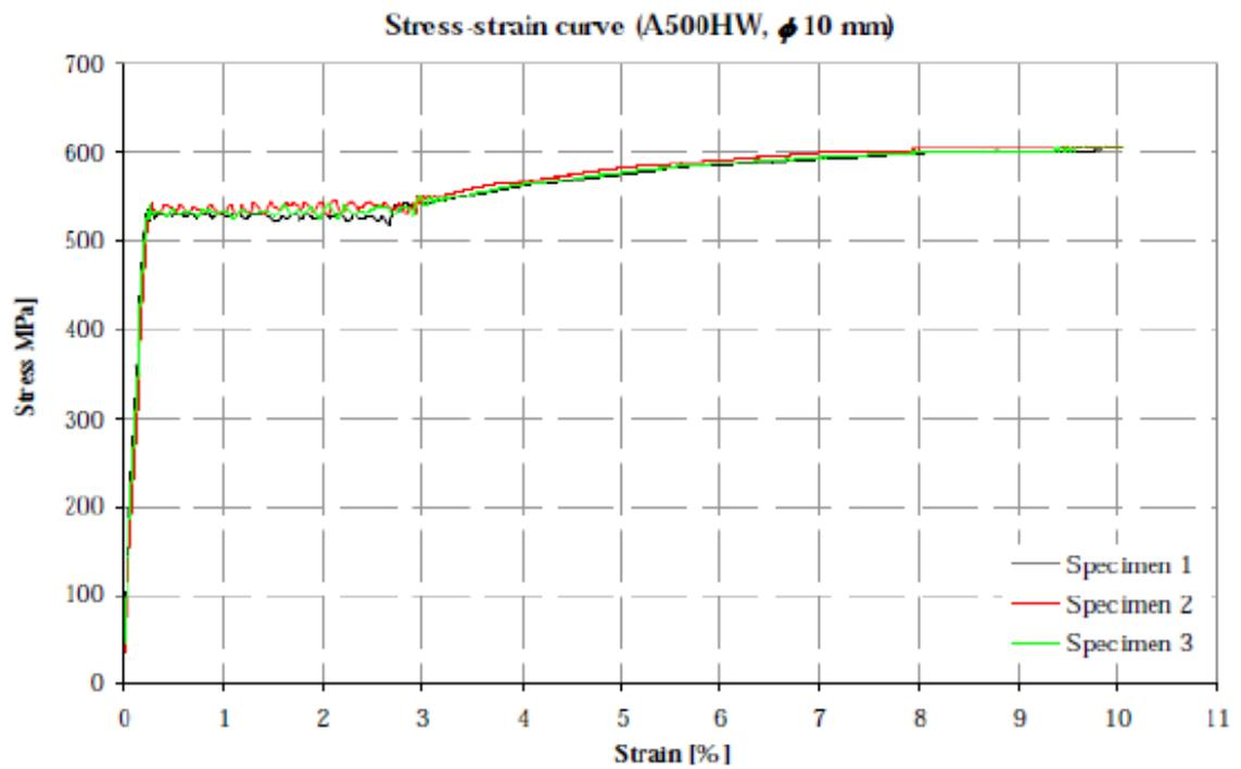
Figure 3.3: Stress-strain curve for A500HW 10mm steel rebar
