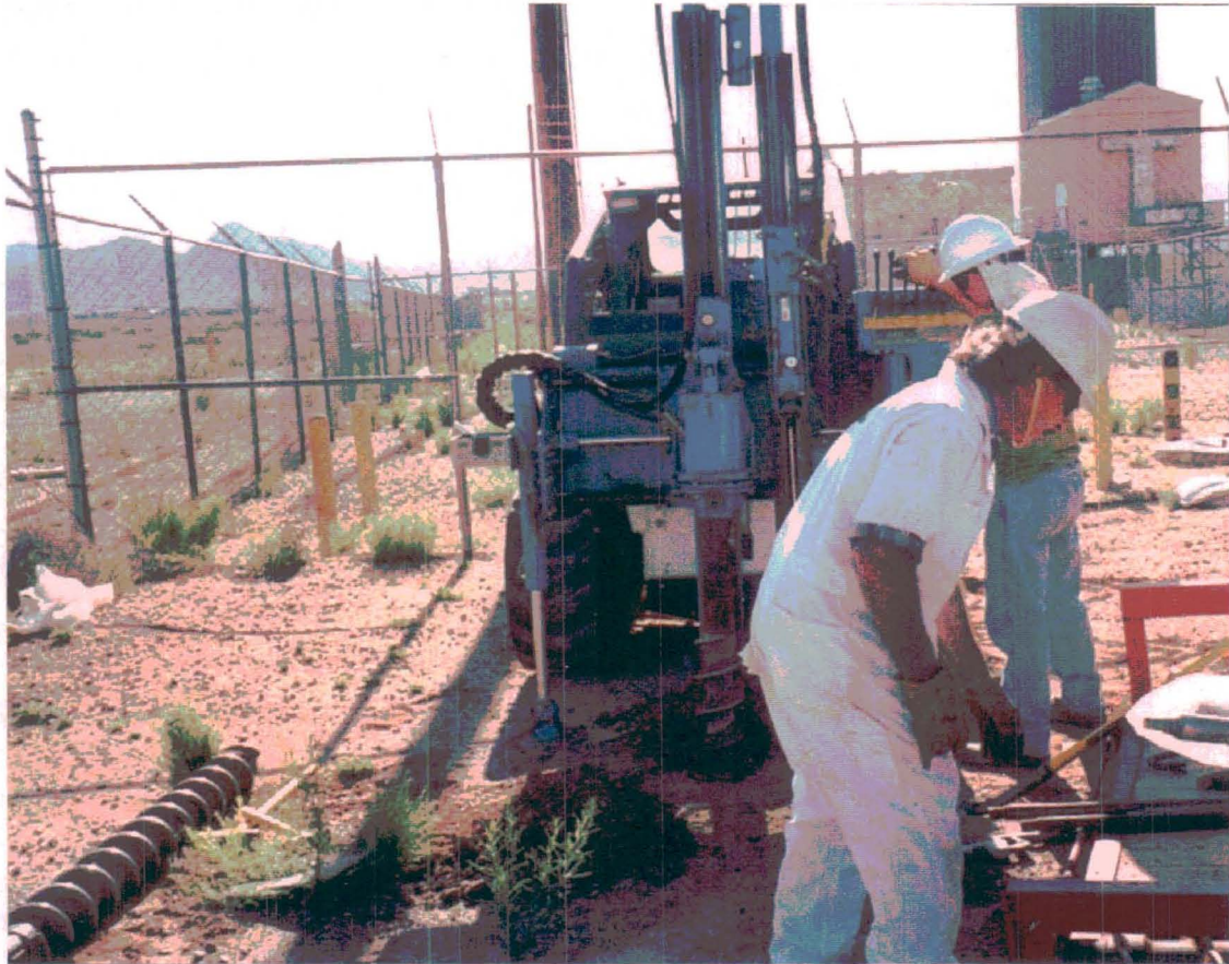
Figure 3.4-2 Collecting soil samples in the DSS Site 1007, Former Building 6730 Septic System Drainfield. View to the east. August 17, 1999
