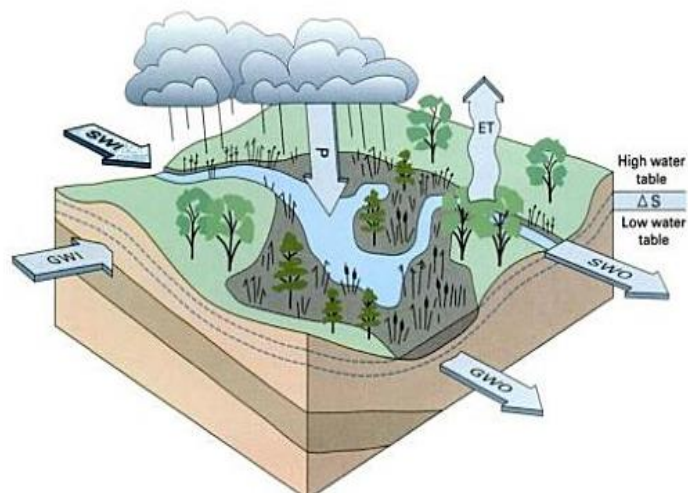
Figure 32: Hydrologic process of wetlands (Carter, 1996)
