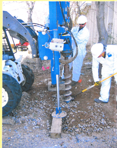
Collecting soil samples with the Geoprobe
