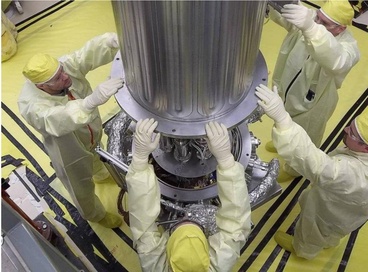
Figure 2.2. KRUSTY experiment with vacuum chamber [12]
