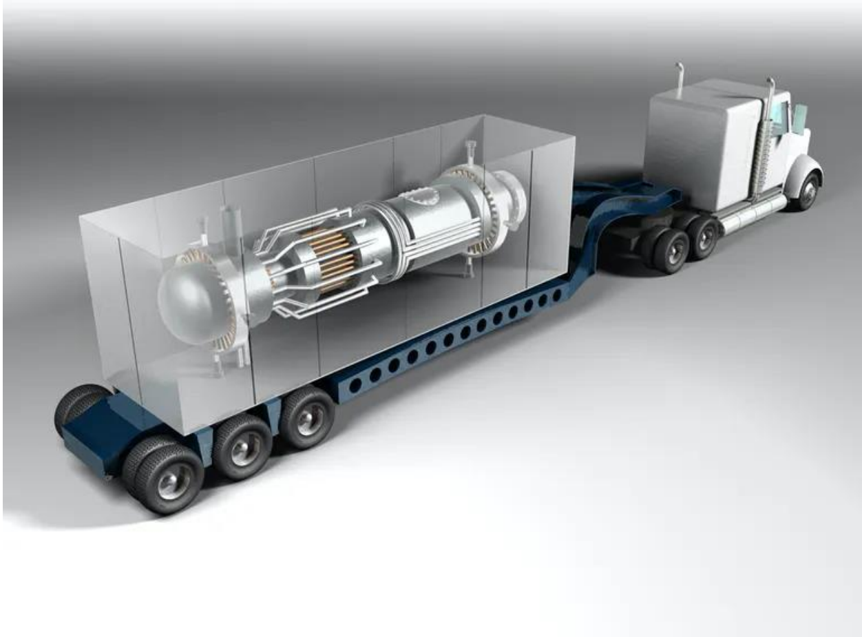
Figure 2.1. Conceptual microreactor hauled by semi-trailer truck [7]
