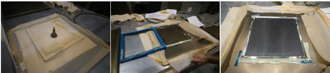
Figure 3.12: Debaggging of cured composite plate.
