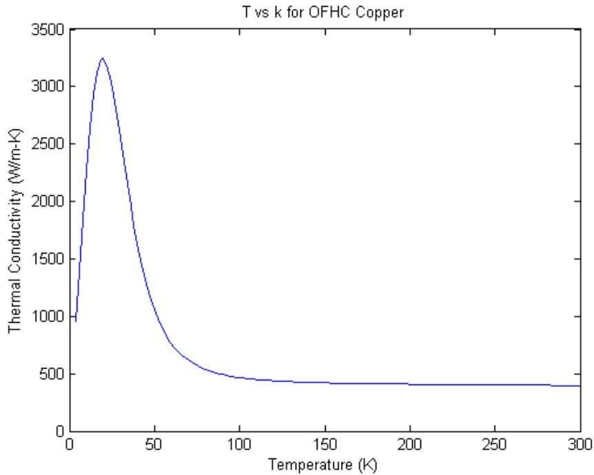
Figure 39: Thermal Conductivity vs Temperature for Oxygen Free Copper
