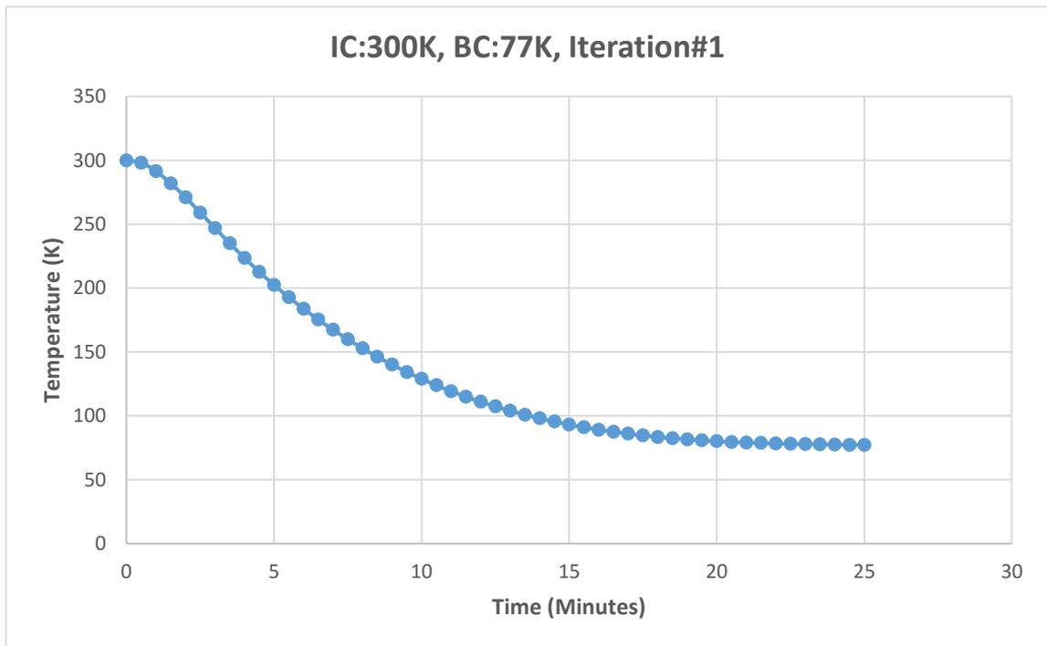
Figure 41: Cool Down Test, Case 1,  $t_{Block}=0.75''$ ,  $L_{Neck}=1.5''$
