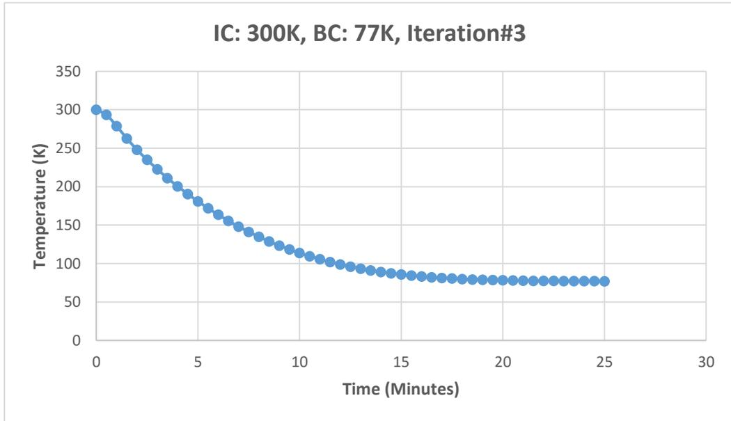
Figure 50: Cool Down Test, Case 1,  $t_{Block}=0.375''$ ,  $L_{Neck}=1.4''$
