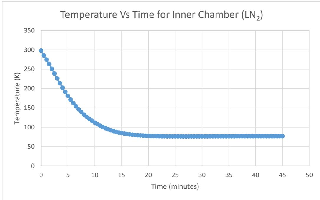
Figure 18: Temperature vs Time for Inner Chamber – Case 1
