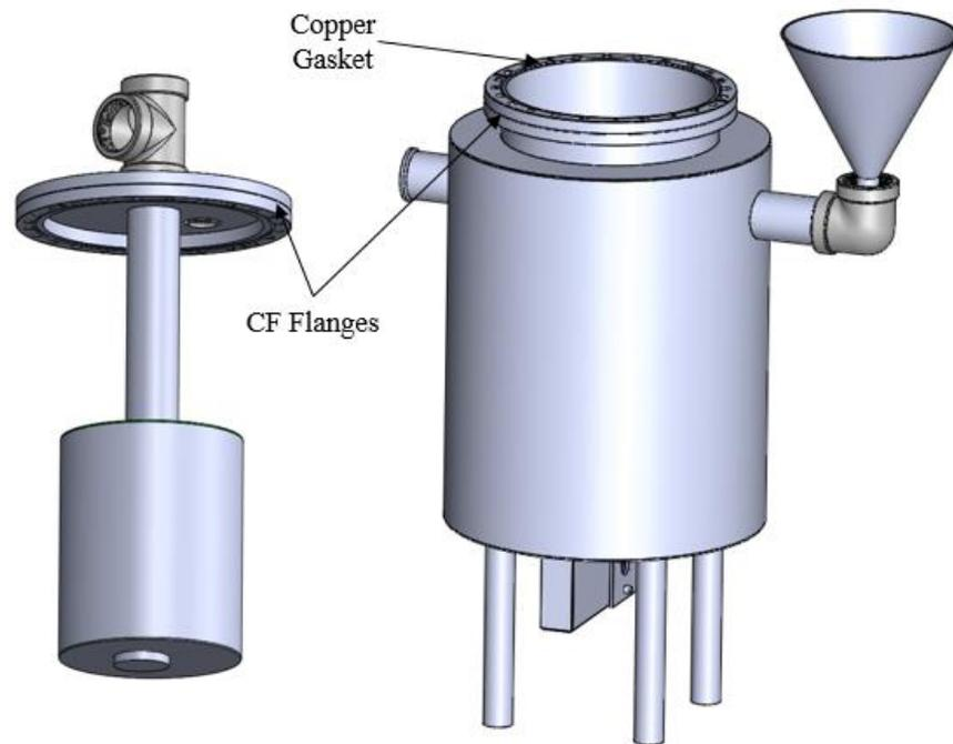
*Figure 28: Separable Parts for the Cryostat*
