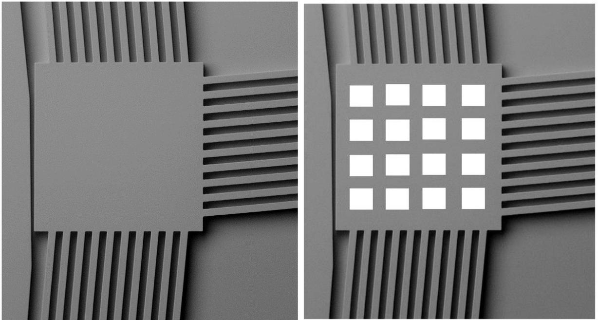
*Figure 85: (Left) Present Chevron Junction (right) Improved Junction*
