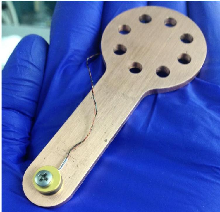
*Figure 33: Copper Arm with Silicon Diode Temperature Sensor*
