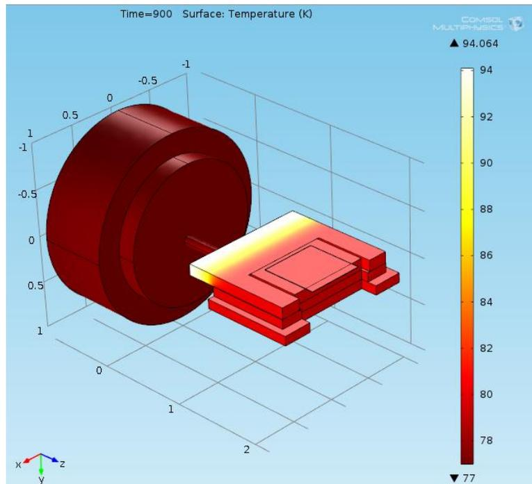
Figure 43: Temperature Distribution at 900 sec, Case 1,  $t_{Block}=0.75''$ ,  $L_{Neck}=1''$
