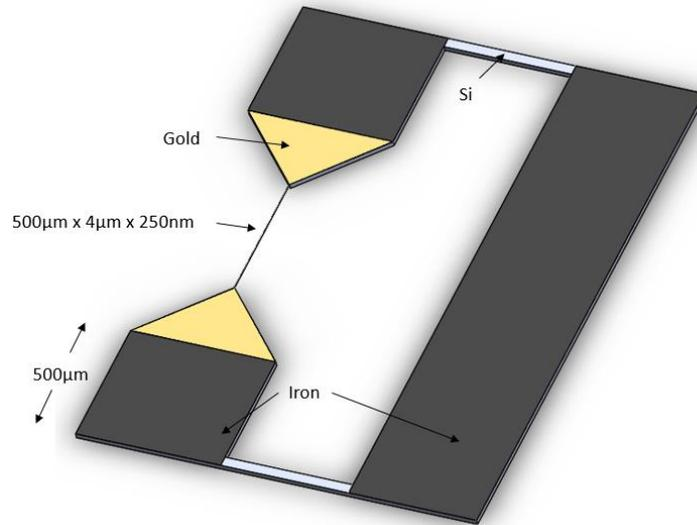
Figure 72: Novel Concept for Transferring Samples through Electromagnetism
