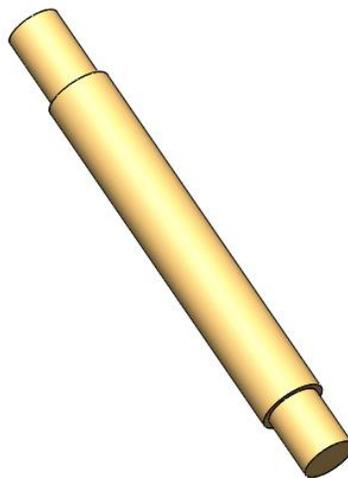
*Figure 61: Separated Holder Neck for Variable Length*
