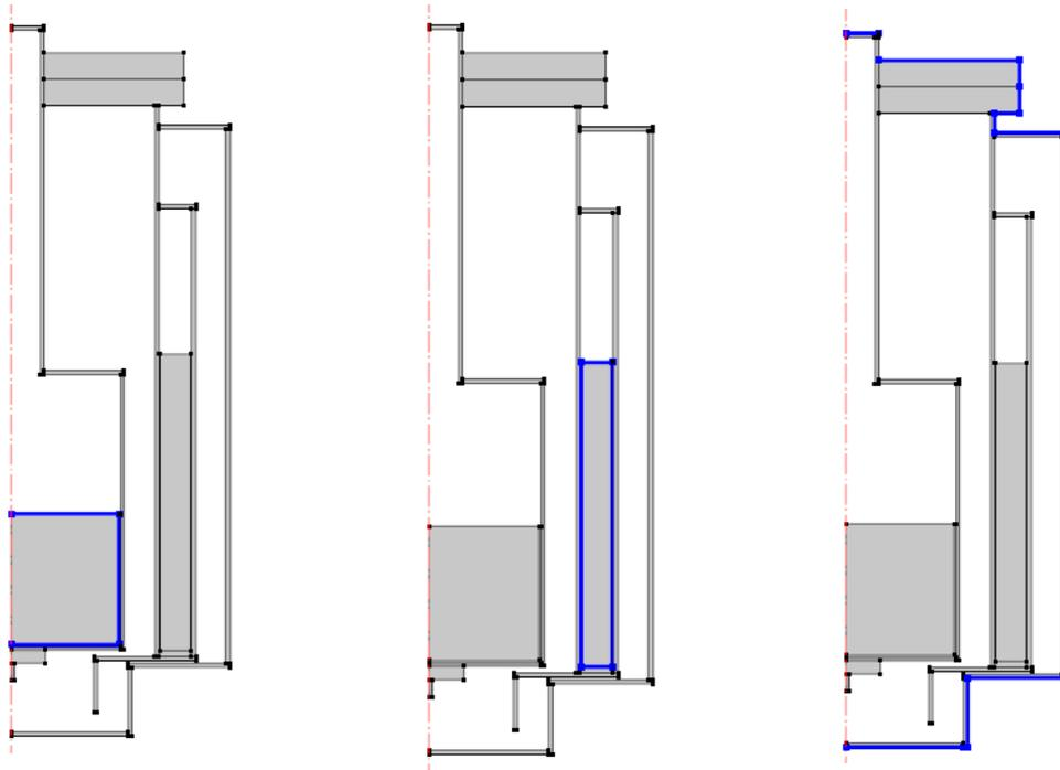
Figure 22: Boundary Conditions for Case-2, (Left to Right) a) Fixed Temperature boundary of 77 K at 99% volume, b) Fixed Temperature boundary of 4.5 K at 99% volume, c) Inward Heat Flux of 10 W/inch<sup>2</sup> and Tambient = 300K
