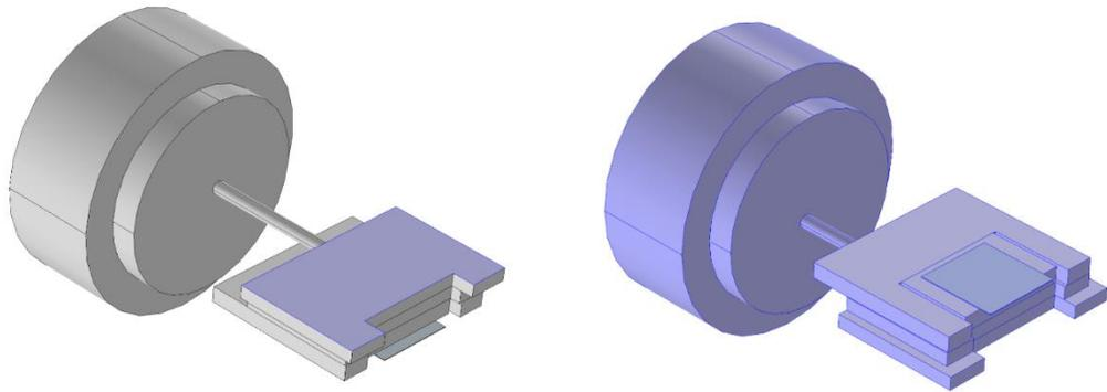
Figure 45: (Left) 10 W/inch<sup>2</sup> Boundary Condition (Right) 77K Initial Condition for Heat Up Test, Case 1
