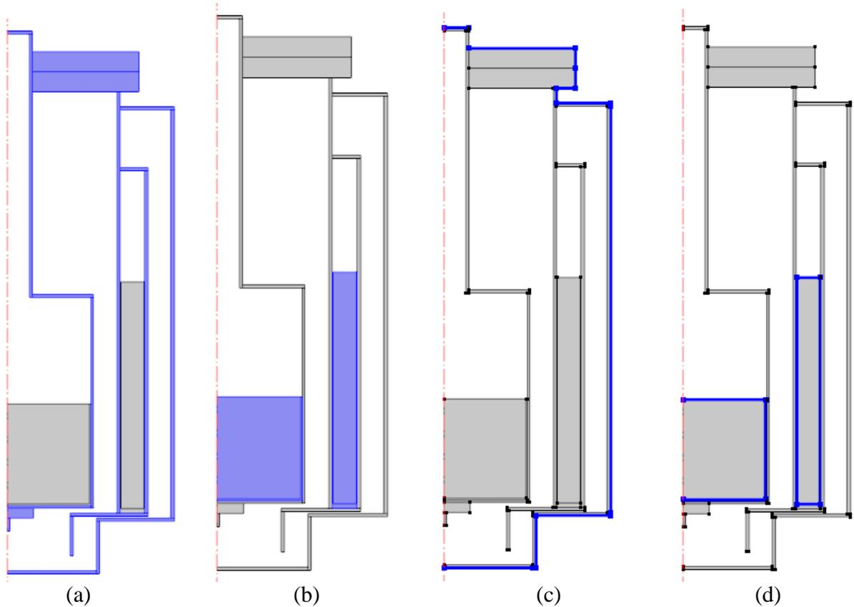
*Figure 8: Initial Conditions for case 1 a) 300K, b) 77K, Boundary Conditions for Case1 c) 10W/inch<sup>2</sup>, 300K inward Flux, d) 77K fixed temperature (Similar to figure 7)*
