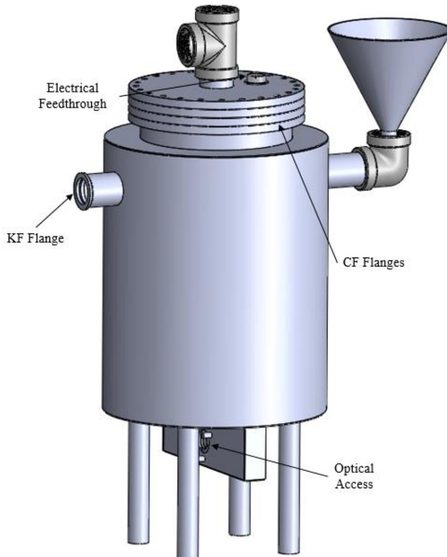
Figure 26: Cross Sectional View of Cryostat
