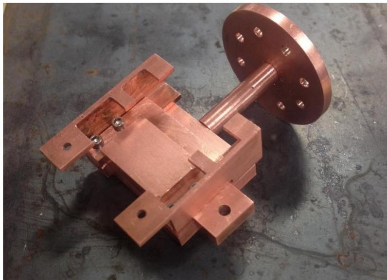
*Figure 63: Assembled Copper Structure of Holder*
