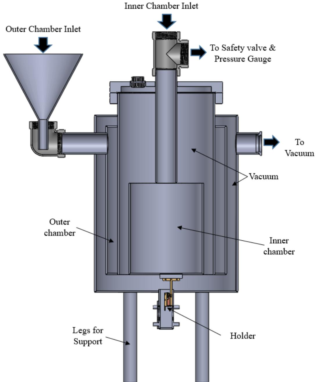
Figure 27: Cross Sectional View of Cryostat
