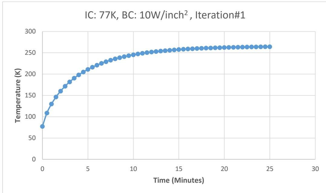
Figure 46: Heat Up Test, Case 1,  $t_{Block}=0.75''$ ,  $L_{Neck}=1''$
