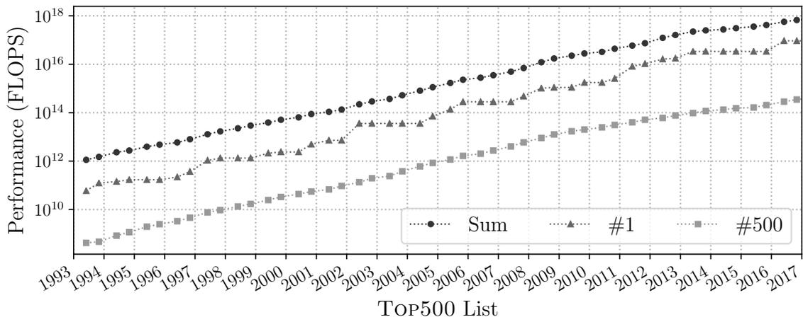
Figure 2.2: Performance development of HPC systems as recorded by the TOP500.
