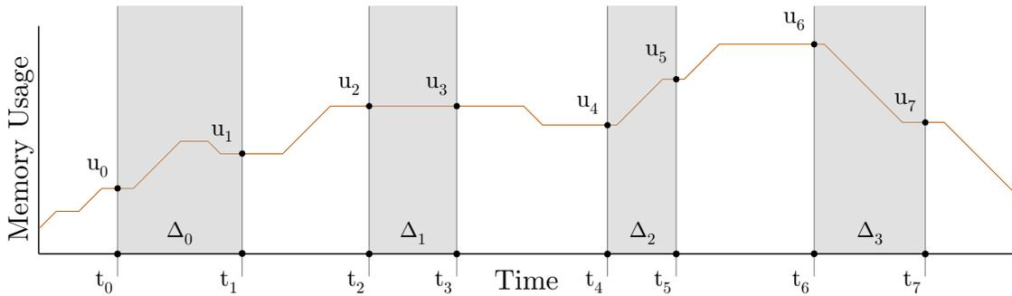
Figure 4.5: Single-process memory usage and data collection points.
