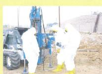
Photograph showing soil sample collection with the Geoprobe at SWMU 105. (Workers are in level C personal protection equipment and monitoring with the MVA.)
