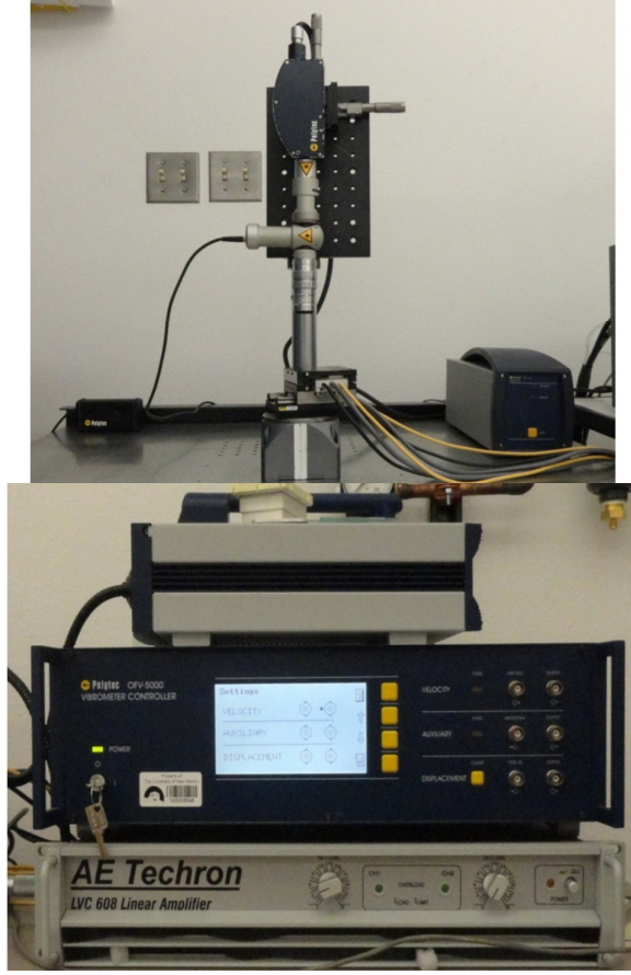
Figure 5.2 Laser Doppler Vibrometer setup. It is fed by laser source from the top and the controller which is connected to X-Y stage presented
