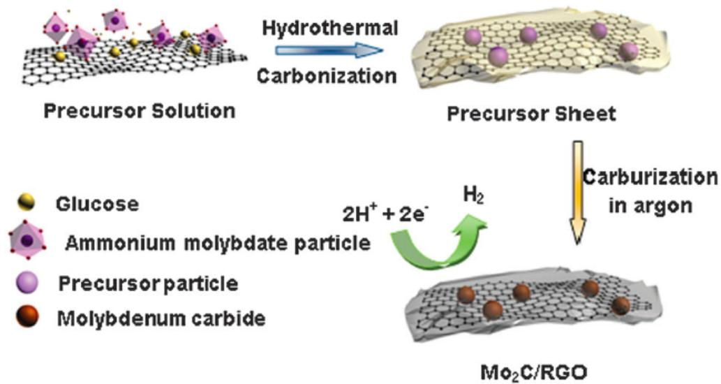
Figure 1-22. Schematic for synthesizing molybdenum carbides reported by Pan *et al.* (34).
