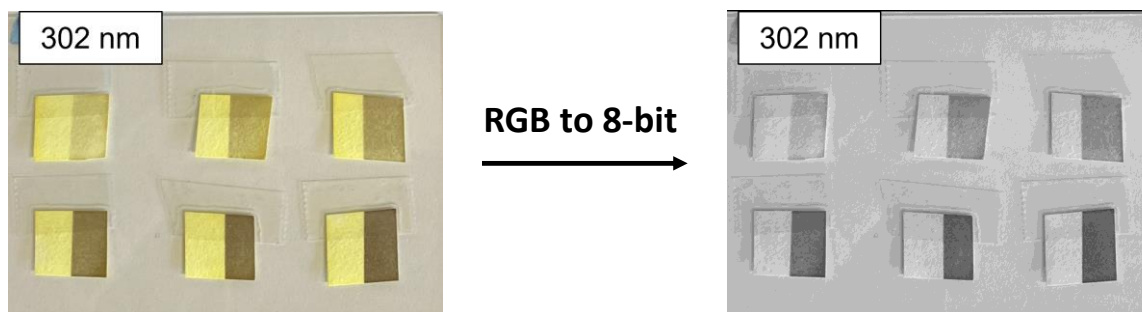
Figure 6.6. 8-bit gray scale conversion of 302 nm solid-state sensor image.
