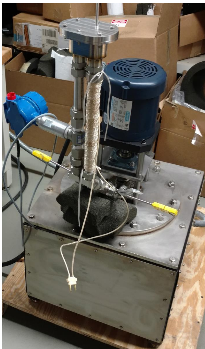
Figure 3-11 Pump and Melt Tank
