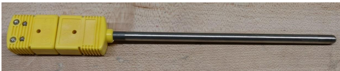
Figure 3-13 1/4" Diameter Omegaclad K-type thermocouple
