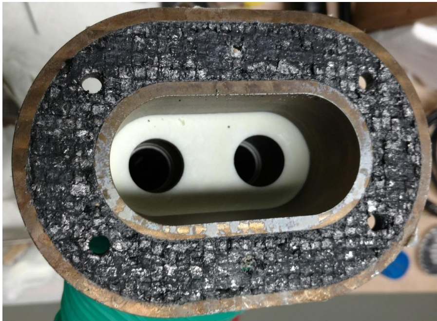
Figure 3-27 Post test expansion tank interior and gasket
