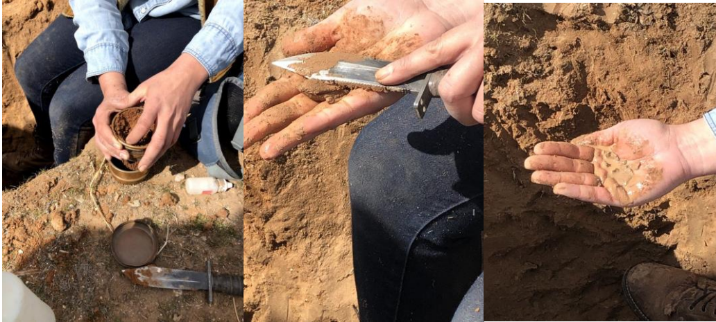
Figure 1. A series of photos garden managers learned about examining physical properties of the soil. Pictured is a consultant inside of a pit to give a demonstration on how to 1) sift particles of soil, 2) work water into the soil and 3) to examine the proportions of clay and silt in the soil (Photo credits: Stefany Olivas).
