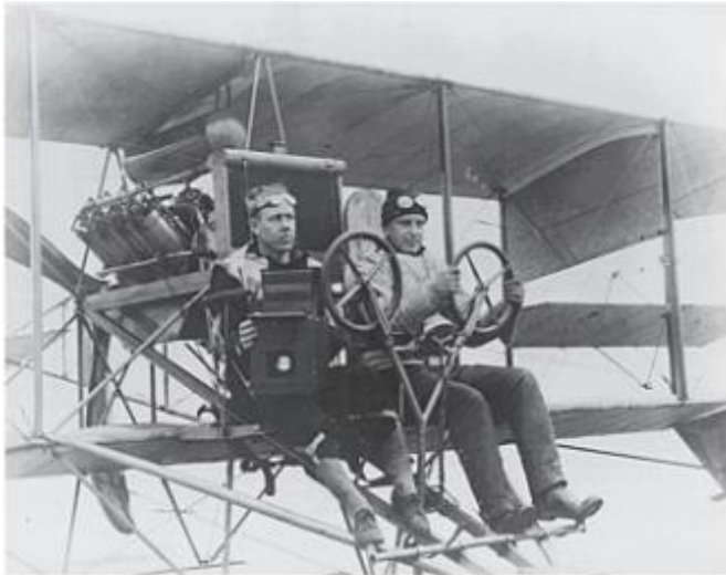
Figure 2.1 A pilot and photographer from the U.S. Navy mounted on an airplane in 1914. “This photograph illustrates difficulties encountered in early efforts to match the camera with the airplane - neither is well-suited for use with the other.” (Campbell and Wynne 2011).
