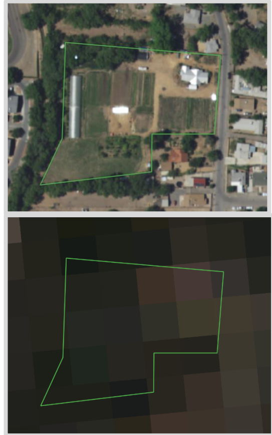
Figure 4.2. Aerial views of the same local farm from NAIP aerial imagery at 1 meter (top) versus Landsat satellite imagery at 30-meter resolution (bottom). Note the clarity of the images, with plot design distinguishable in the NAIP image (U.S. Geological Survey 2022).
