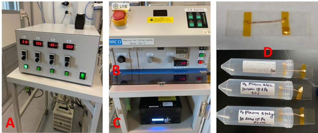
Figure 22: Reactive ion etching setup and samples: (A) Gas supply, (B) Etching chamber, (C) RF generator, (D) Sample preparation.
