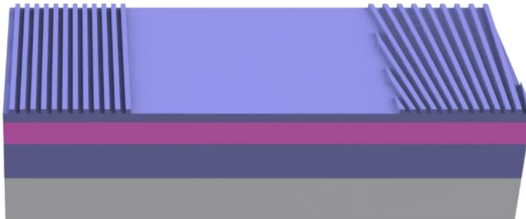
Figure 3-8: schematics of chirped grating spectrometer. The chirped grating region is across 16mm width. For the present experiments, the propagation region is 1.2 cm long to allow for mounting of the commercial detector array.
