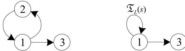
Figure 1.5: Basic elements for flowgraph analysis: loop, reduced loop
