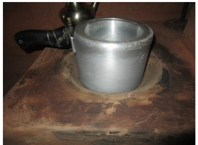
Figure 8: Pot fits efficiently on the Rayali ICS in Figure 6
