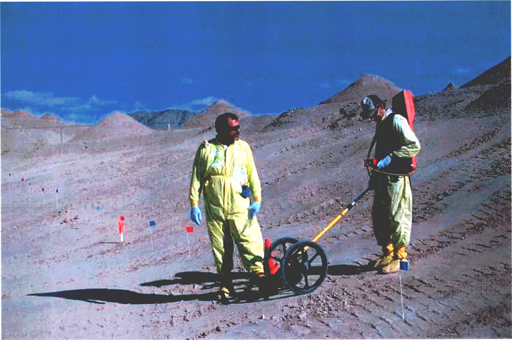
Figure 5.7.1-1 Geophysical Surveying in the SWMU 2 Excavation
