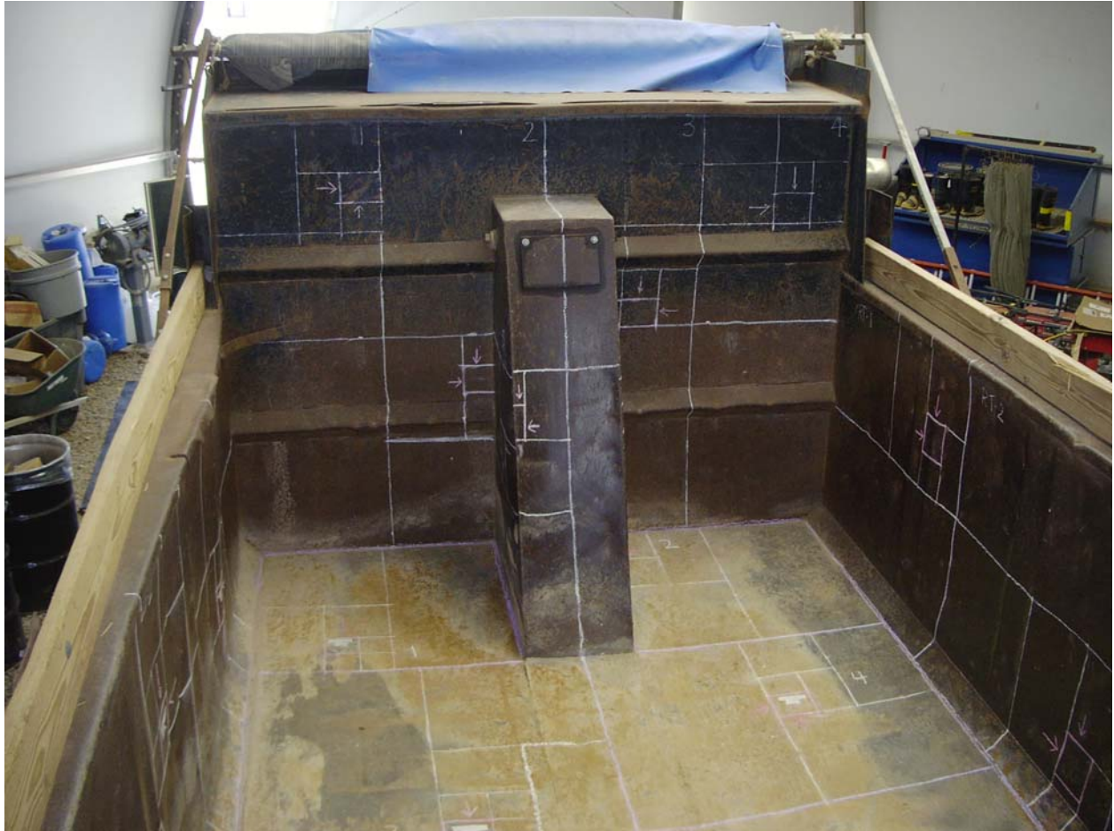
Figure C-4 Dump Truck PCB Wipe Locations, September 3, 2003
