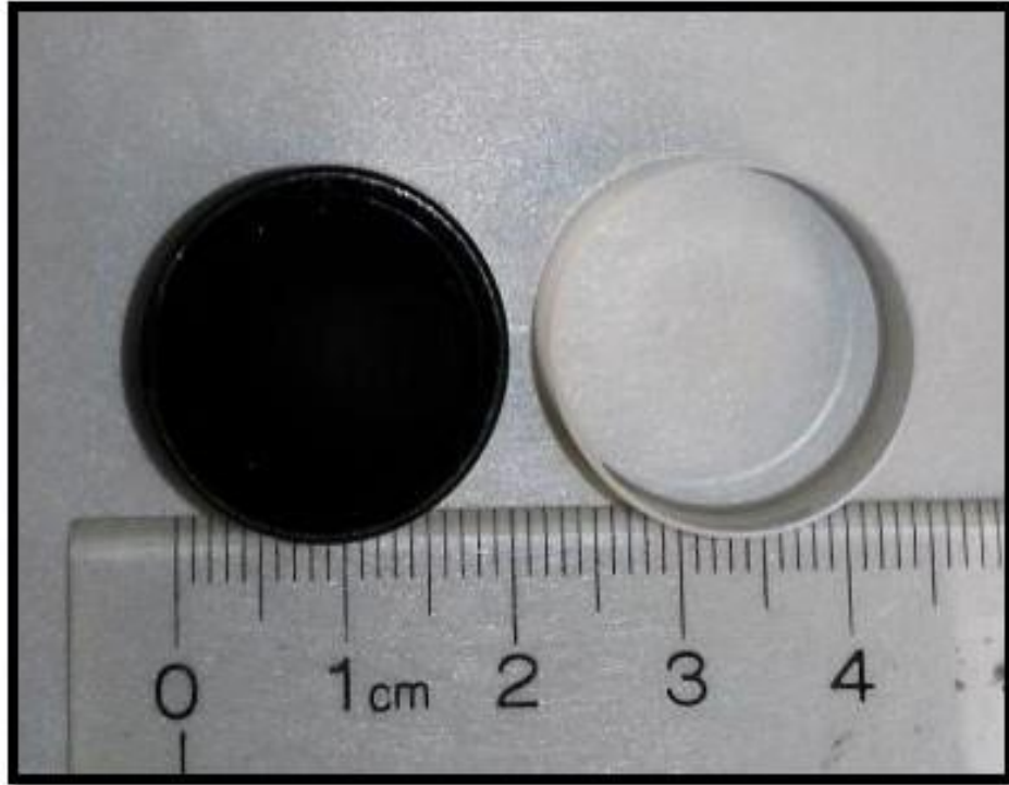
Figure 5.6.1: Side-by-side comparison of the OSU irradiated sample B15-5 and the non-irradiated control sample B15-1. This photograph demonstrates a darkening in the crystal due to the harsh environment of the OSU TRIGA reactor.
