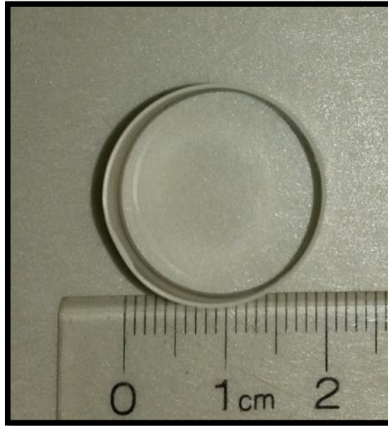
Figure 3.2.8: Picture of a \text{CaF}_2 FPE utilized in this research. This FPE is the 20.3 mm diameter sample.
