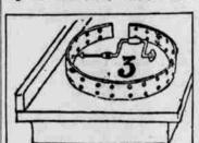
Fig. 3-Countersinking the Holes in the Brake Band.
