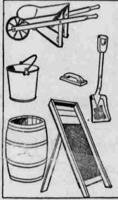
Simple Tools for Making and Placing Concrete: Water Barrel and Bucket; Steel Pan Wheelbarrow for Handling Dry Aggregate, and Hauling Concrete to Forms: Sand Screen for Proper Grading of Aggregates; and Mixing Concrete, and Wooden Float for Finishing.
