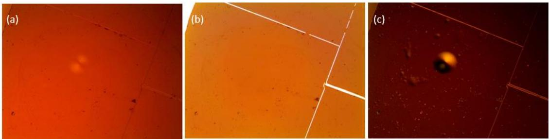
Figure 3.10 Optical microscope images of the bonded sample on a substrate from the top in reflection (a), transmission (b), and Normaski (c) modes. The field of view is about 0.7 mm by 0.5 mm. There are cracks (straight lines), interface bubbles, and black wax residues on the sample.
