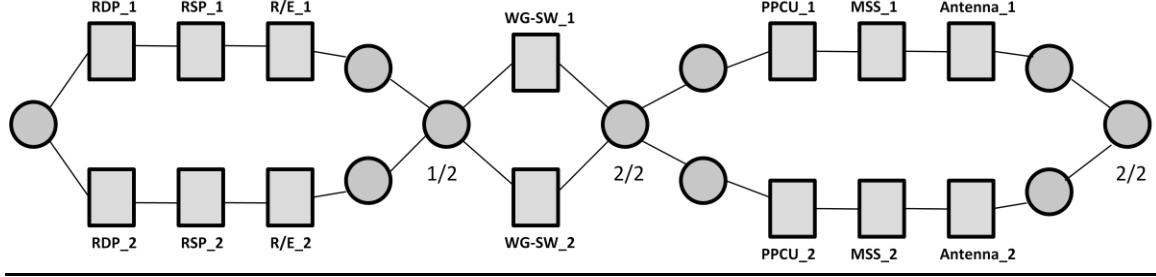
**Figure 5:** B-2 RMP (Radar Modernization Program) Reliability Block Diagram
