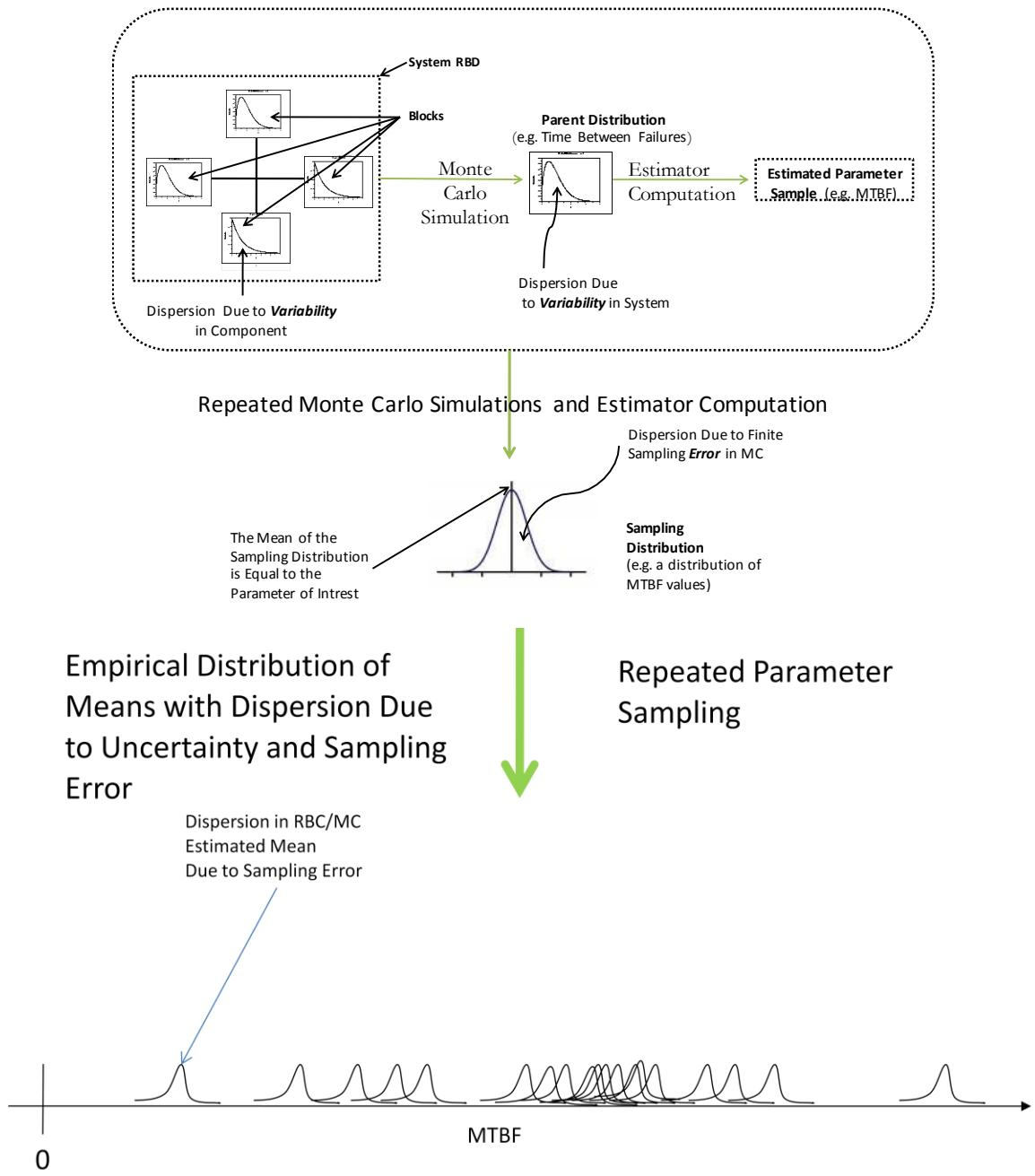
**Figure 4:** Depiction of the system-level uncertainty analysis conducted by applying an extra layer of sampling from parameter distributions
