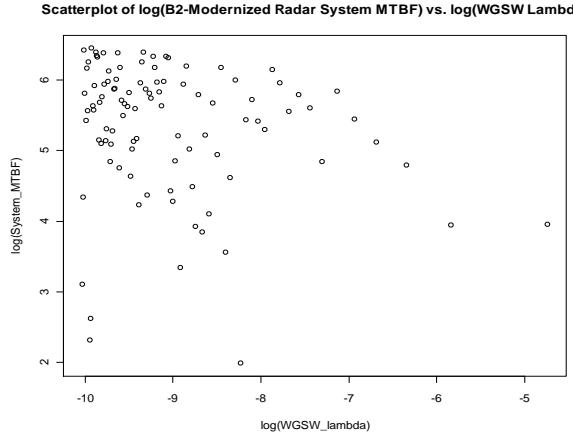
**Figure 6:** Scatterplots of  $\log_e(\text{System MTBF})$  vs.  $\log_e(\lambda_i)$ , for  $i = 1, 2, \dots, 7$  for each of the seven redundant structures
