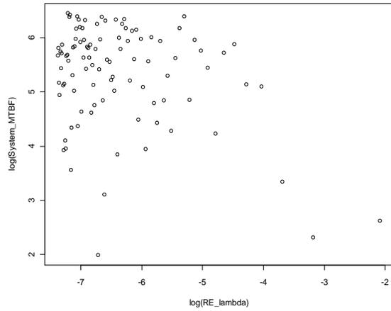
Scatterplot of log(B2-Modernized Radar System MTBF) vs. log(RSP Lambda)
