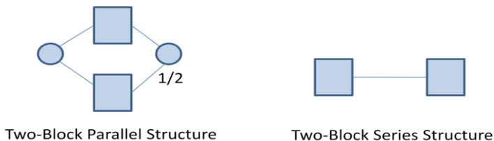
**Figure 1:** Basic Recursive Structures in an RBD
