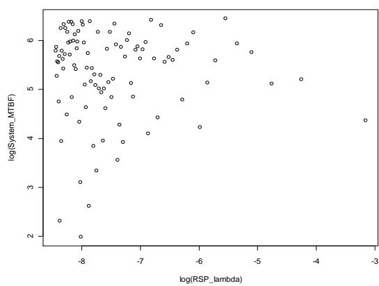
Scatterplot of log(B2-Modernized Radar System MTBF) vs. log(RDP Lambda)
