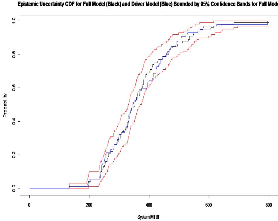
**Figure 12:** Plot of system uncertainty CDF for the full model (black) and the driver model (blue) bounded by 95% point-wise confidence bands estimating sampling error in full model MTBF determination.
