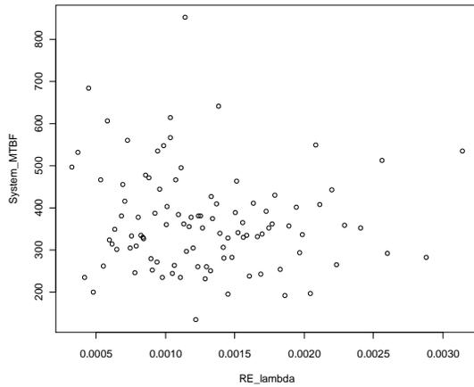
Scatterplot of B2-Modernized Radar System MTBF vs. Antenna Lambda
