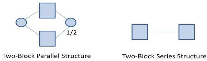
**Figure 1:** Basic Recursive Structures in an RBD
