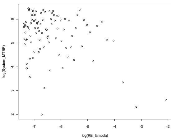
Scatterplot of log(B2-Modernized Radar System MTBF) vs. log(RSP Lambda)
