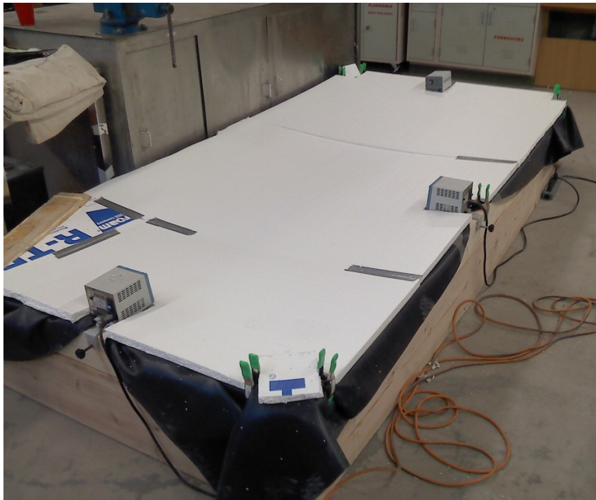
Figure 3.28: UHPC curing tank
