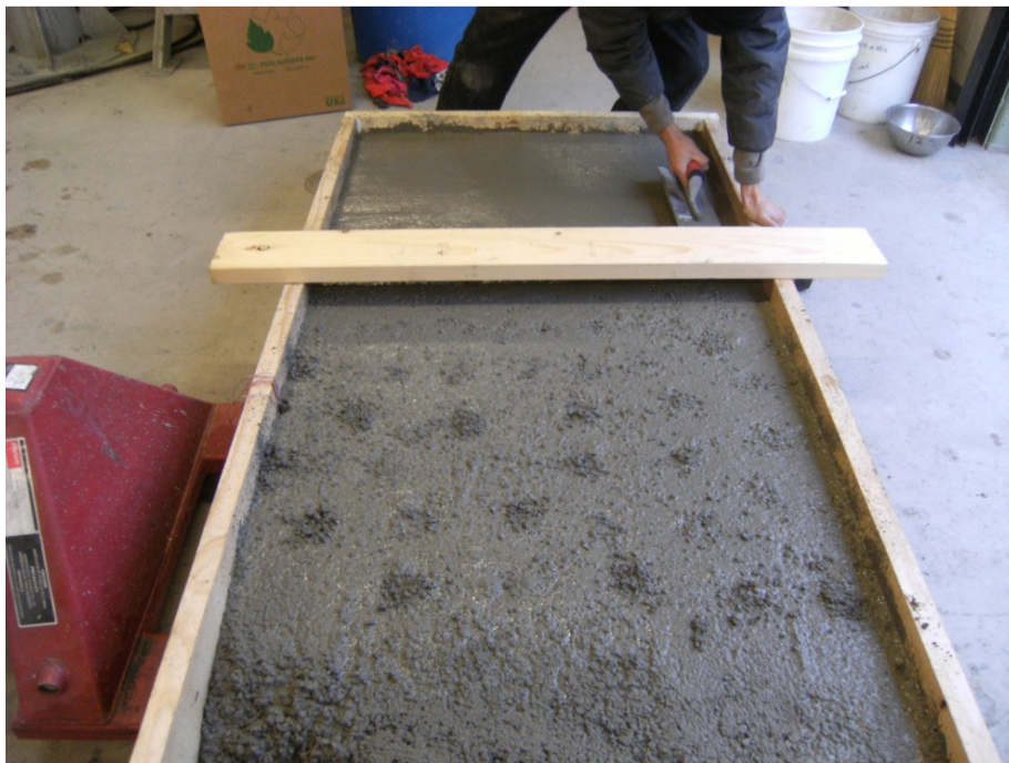
Figure 3.14: Finishing the control slab
