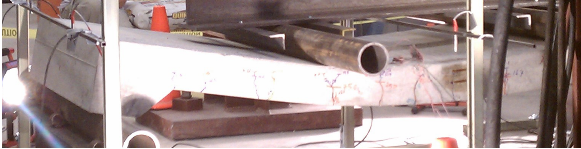
Figure 5.2: Deflection of the control slab near failure
