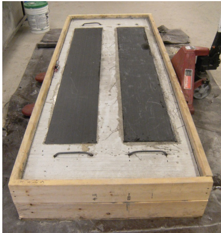
Figure 3.23: CFRP and shear-friction reinforcement
