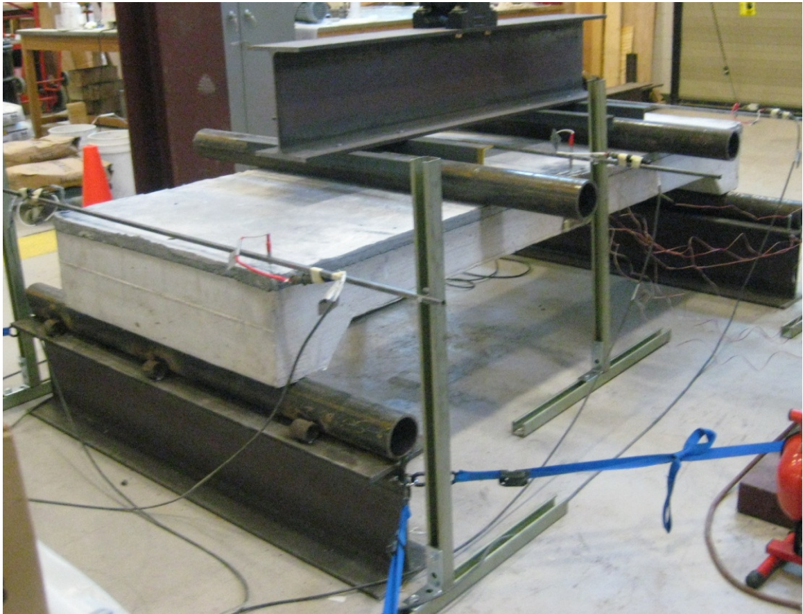
Figure 3.34: The strengthened slab prior to testing
