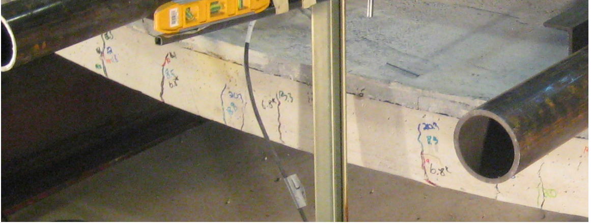
Figure 5.22: UHPC and NVC slab prior to buckling
