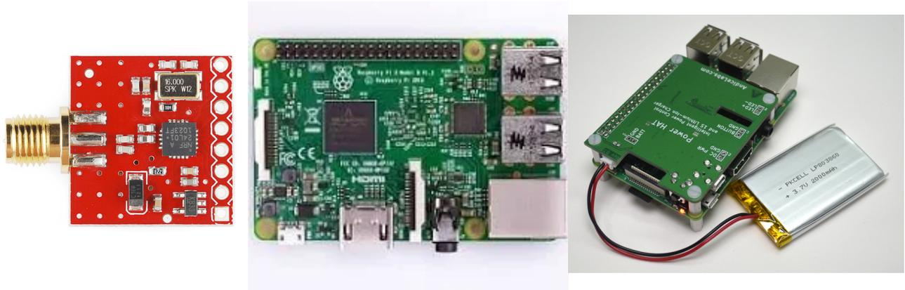
Figure 4: Hardware used for the fire fighter nodes and the relay points to be placed as standalone transceivers.
