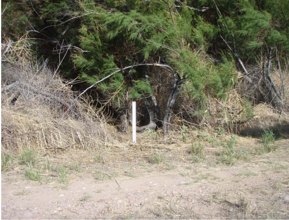
Photo 23: A staff gage installed on the east slope of the Bosque del Apache Levee for monitoring the water surface during the 2008 spring runoff. Foreground is the top of the levee (May 2008, Rolland)
