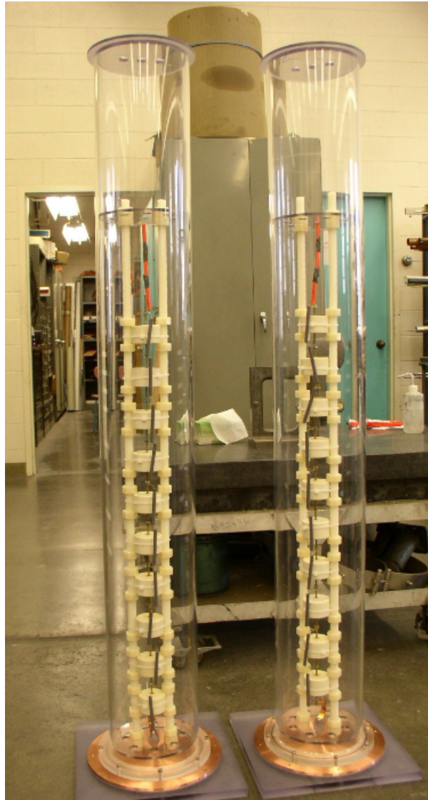
Figure A.2: Container for the 300-kV capacitor bank.
