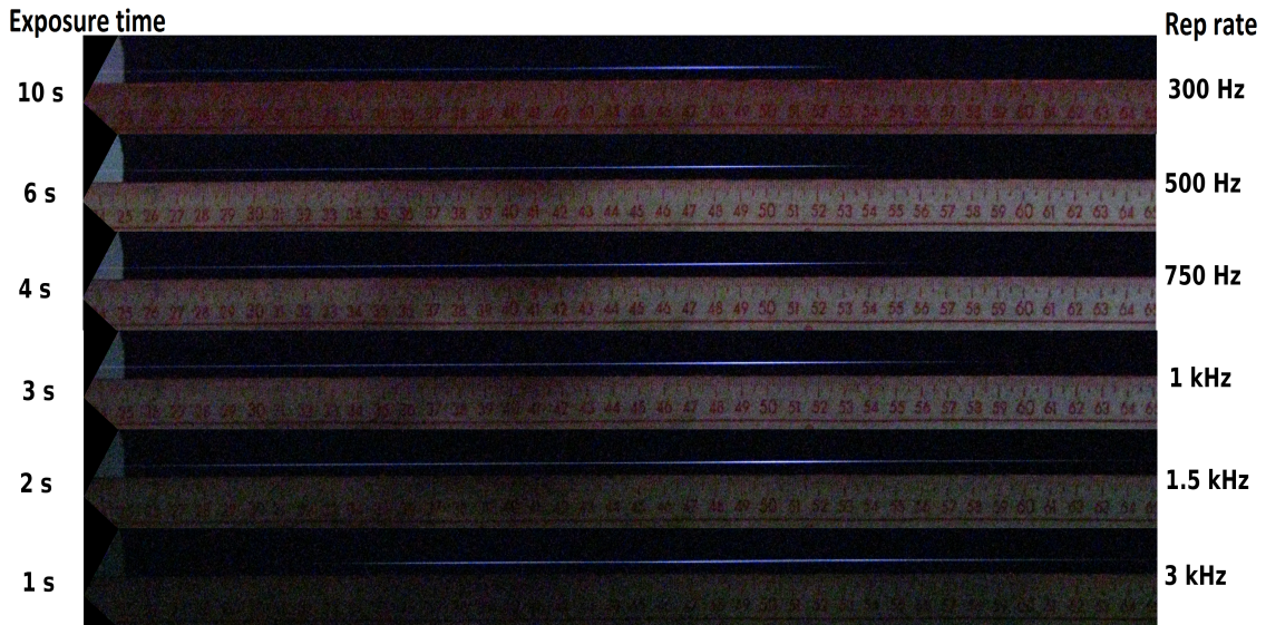
Figure 4.5: Images showing the length and position of a filament’s region of brightest ionization at different repetition rates using a digital camera. The laser propagated from left to right starting at the 24.5-cm mark on the left to the 65-cm mark on the right. (PM&AM Research, IR&D)
