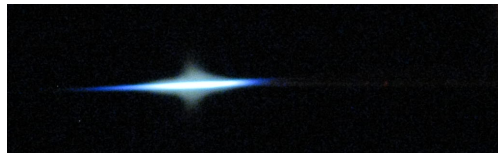
Figure 4.14: Digital photograph of laser plasma in air generated using a 40 fs 1 mJ laser pulse at 5 kHz repetition rate focused by a f = 30 cm lens. The laser propagated from left to right. (PM&AM Research, IR&D)
