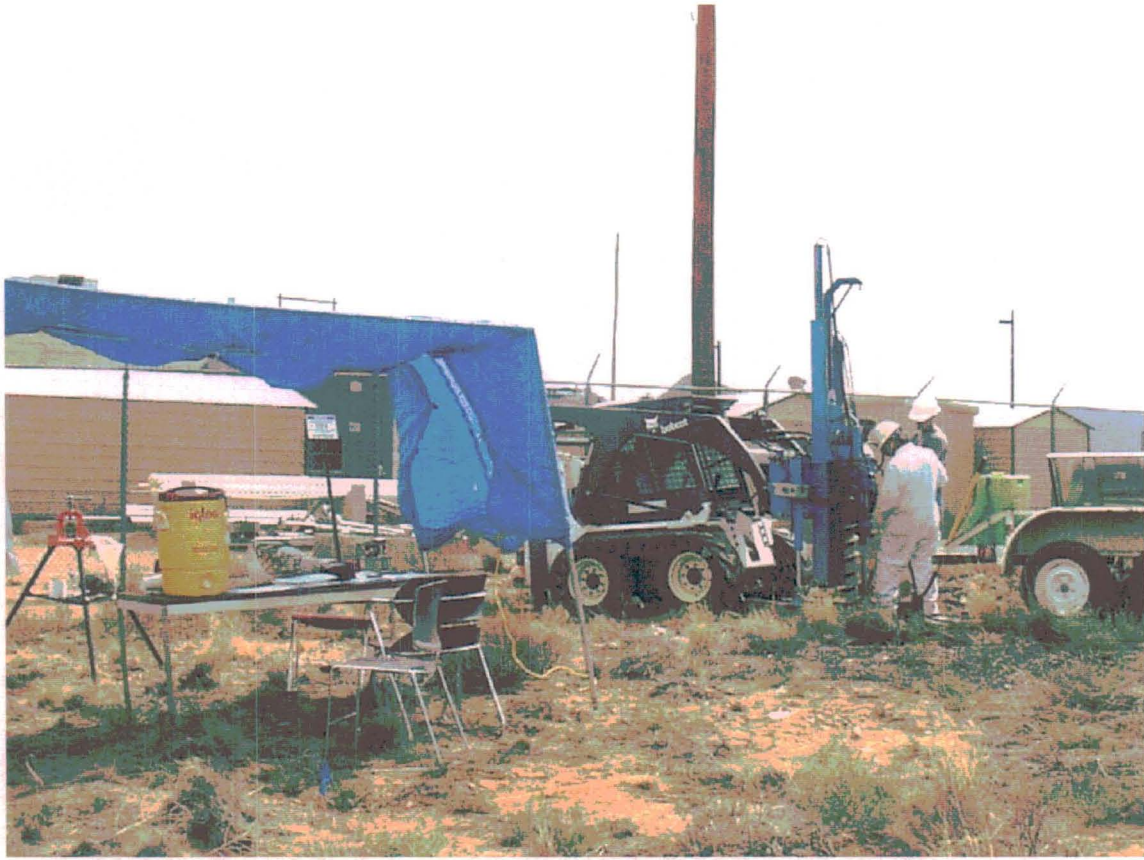
Figure 3.3-1 Collecting soil samples with the Geoprobe™ beneath the west seepage pit at DSS Site 1108, Building 6531. View to the northeast. September 3, 2002
