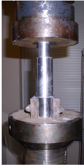
Figure 3.8: Apparatus for compacting discs of C-S-H
