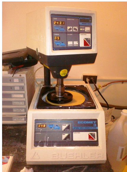
Figure 3.16: Auto-polisher used in preparation of nanoindentation specimens
