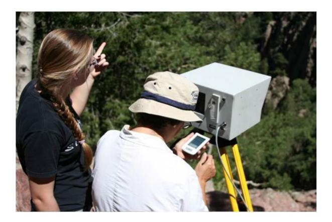
The researchers are using multiple methods to monitor bank stability. One method, Light Detection and Ranging, or LiDAR, is a laser imaging technique capable of resolution up to 1 millimeter. Another method involves placing erosion pins in sets above and below water surfaces. Erosion is determined by measuring how much of the pin is exposed over time. Additionally, the researchers are using a submerged jet apparatus to measure how much different soil types erode.
