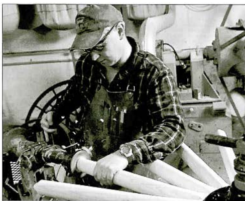
Hansen wheelwright, Tim Hoffman, cutting tenons onto the spokes of a new wheel. (Photo: Hansen)
