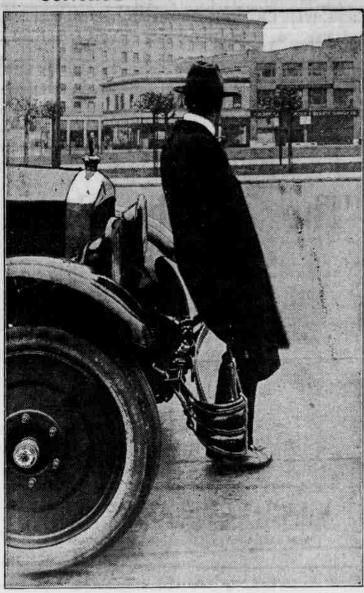
The Illustration Shows the Flexibility of Contact and Bow-Shaped Cushioning Protection Afforded Driver and Object Hit.
