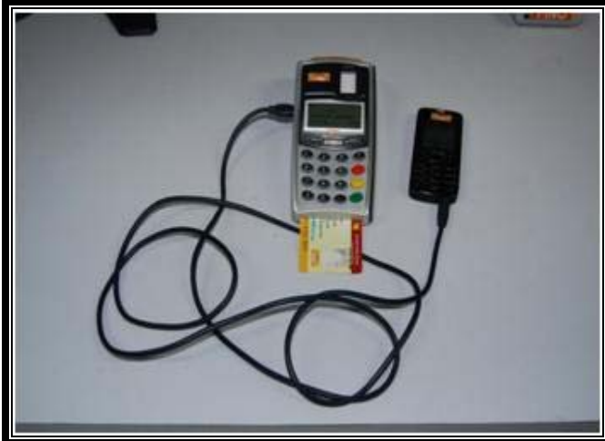
A sample biometric smart card reader; note the card punching place, the GPRS connector and the thumb reader.
