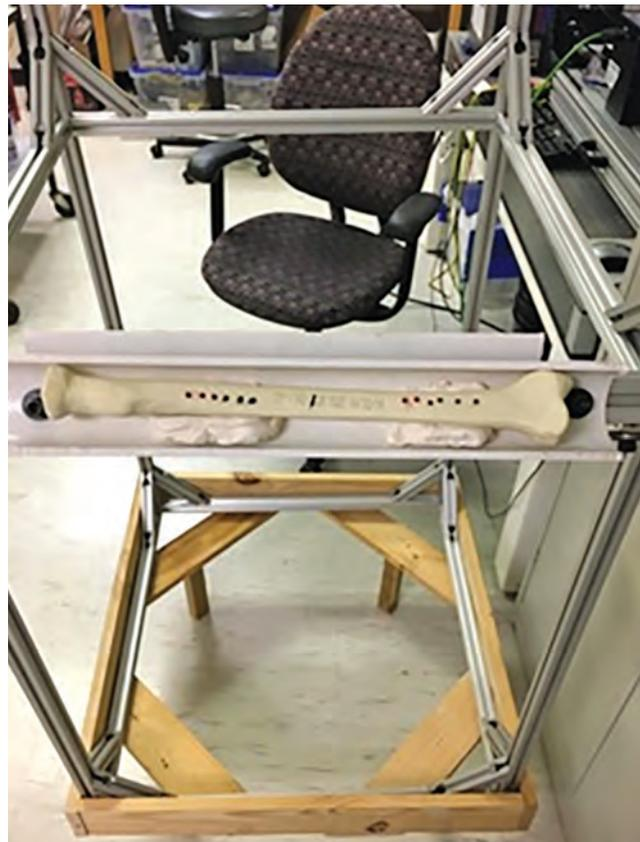
**Figure 2.** Sawbone model in supine position.
