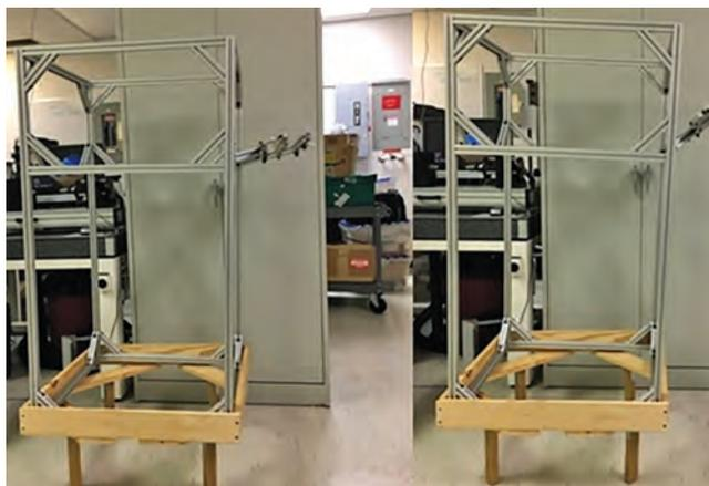
**Figure 1.** Aluminum frame to simulate supine (left) and beach-chair (right) positioning.
