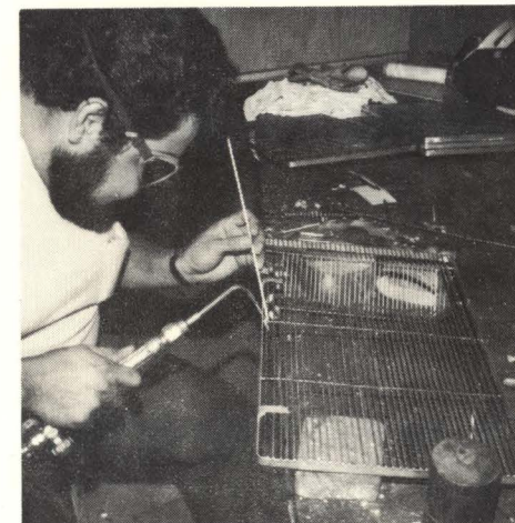
Pictured above is Max Apodaca welding the cages which house the rats that are used for medical research in the Medical School. The Welding Shop repaired about 200 of these cages last year. Larry Forney explained that the rats tug and chew around the edges until the cages start to come apart and then they escape, so periodically the cages have to be repaired.
