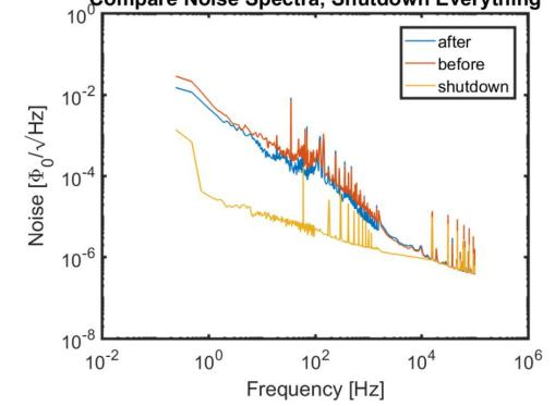
• The first time we ran the new drive electronics, we thought the SQUIDs had gone to the voltage rail and needed resetting (they were so quiet we thought they had stopped working). From the SQUIDs we now cannot tell if
