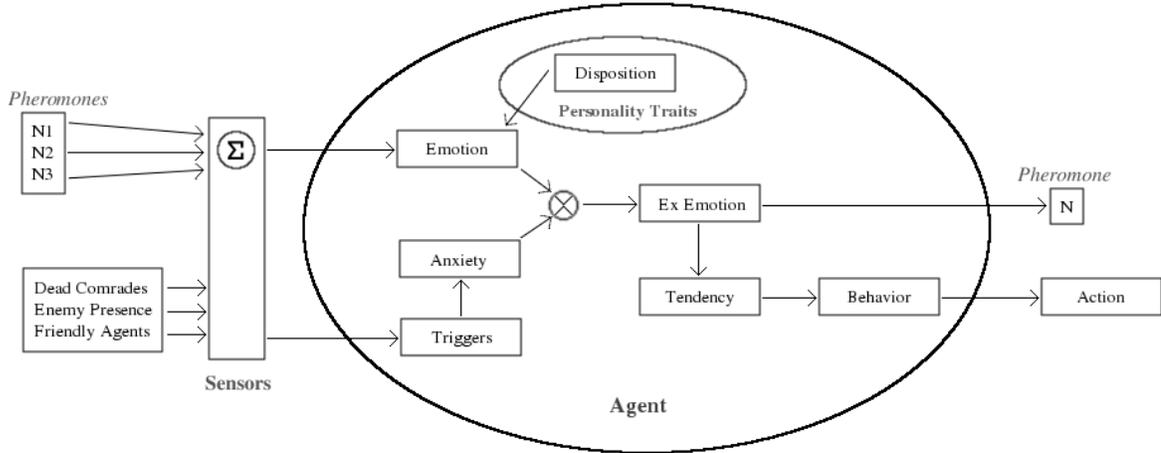
Figure 4: Diagram of Extended-DETT model. The model is implemented in an autonomous agent. Various inputs and internal operations result in not only an action, but also a pheromone that is communicated to other agents.
