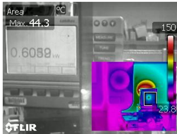
Fig 4.19 MVBGs heating at high input power of 0.6 kW, left corner shows the maximum temperature of 44.3 °C measured within the MVBGs aperture
