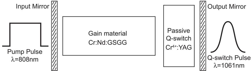
Figure 1.4: Illustration of the basic components of the passively Q-switched lasers studied in this thesis. The laser consists of Cr:Nd:GSGG gain material followed by a Cr<sup>4+</sup>:YAG passive Q-switch. The input and output mirrors are coated directly onto the resonator crystals, creating a flat-flat resonator. The laser resonator is end-pumped by a laser diode at 808 nm and produces a Q-switched laser pulse at 1061 nm.
