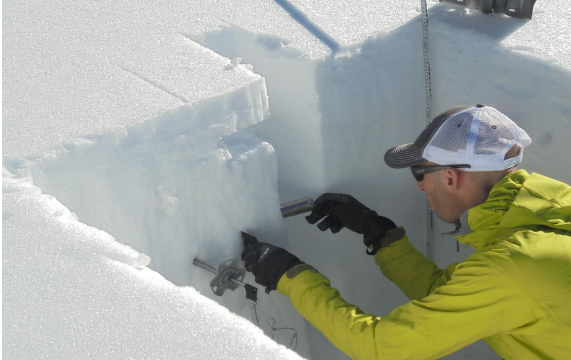
Image 2. Author performing layer density measurements during a snow profile on 2/12. Additional data collected during the snow profile were layer characteristics, grain types and size, and temperatures
