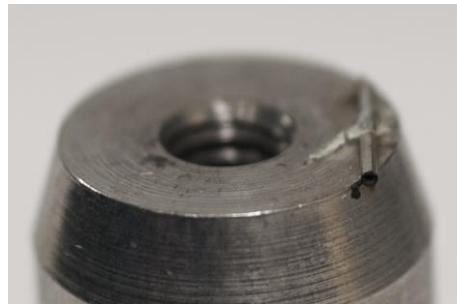
Figure 3.10 Metallic waveguide. Waveguide is glued to a post that is mounted on a 3-axis translation stage.
