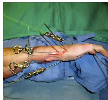
Figure 3: Experimental testing fixture showing trajectory of tendon loading and thumb lateral pinch motion.
