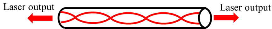
Figure 1.2 Scheme of a Fabry-Perot nanowire laser. A standing wave is formed in the nanowire cavity along the nanowire axis. The end-facets of the nanowire serve as the optical output couplers.
